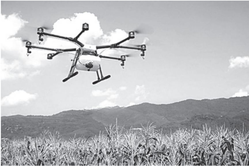
PLATE 7.2 ‘DJI GH-1 Agras’ is a pesticide spraying drone.
