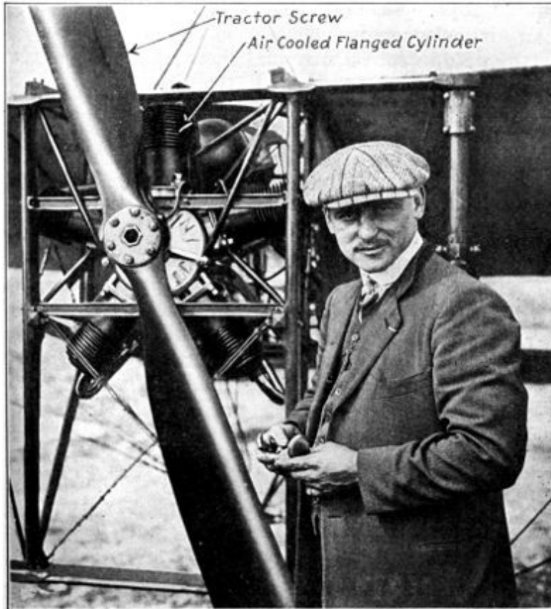
Fig. 85.—Anzani Testing His Five-Cylinder Air Cooled Aviation Motor Installed in Bleriot Monoplane. Note Exposure of Flanged Cylinders to Propeller Slip Stream.
