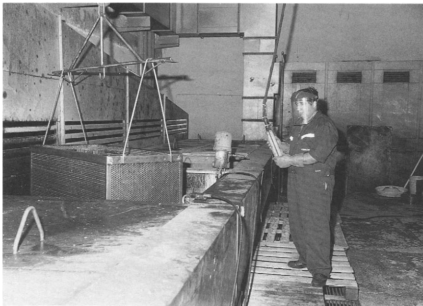
FIG. 11. Treatment of metal surface in the hydraulics shop; The slot hood is seen along the line of baths.
