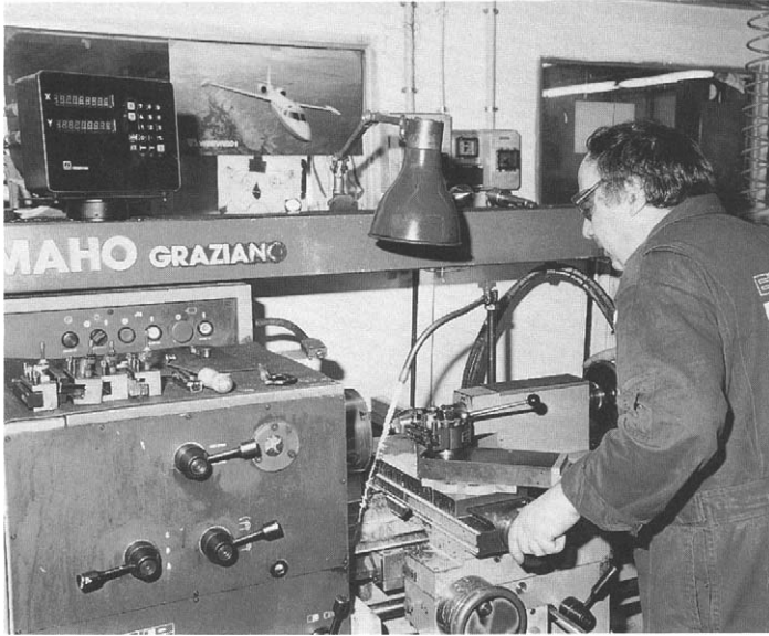
FIG. 6. The lathing process: Oil mist is produced by a constant flow of oil–water emulsion which reduces heat generated by friction. (Note that the worker is not wearing protective gloves.)
