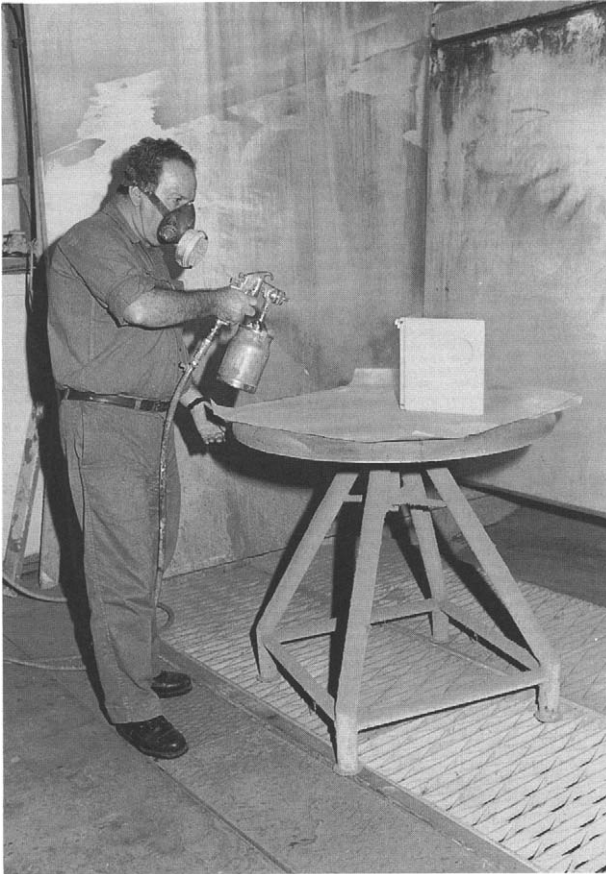
FIG. 7. Spray painting inside a paint booth.
