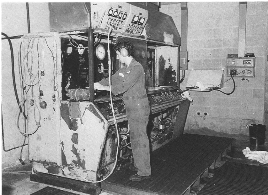
FIG. 14. A setup for testing hydraulic aircraft parts (hydraulics shop).
