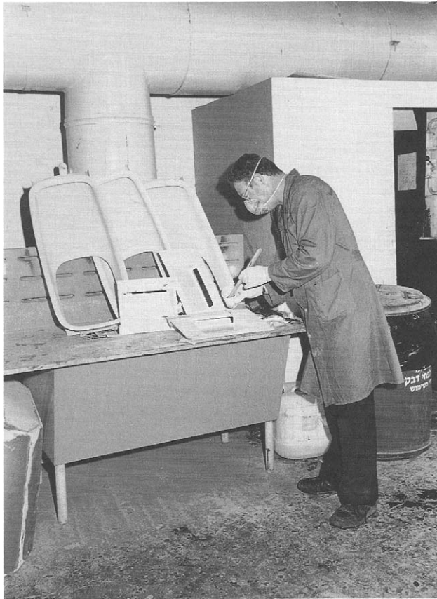
FIG. 8. Epoxy gluing during preparation of a composite structure.
