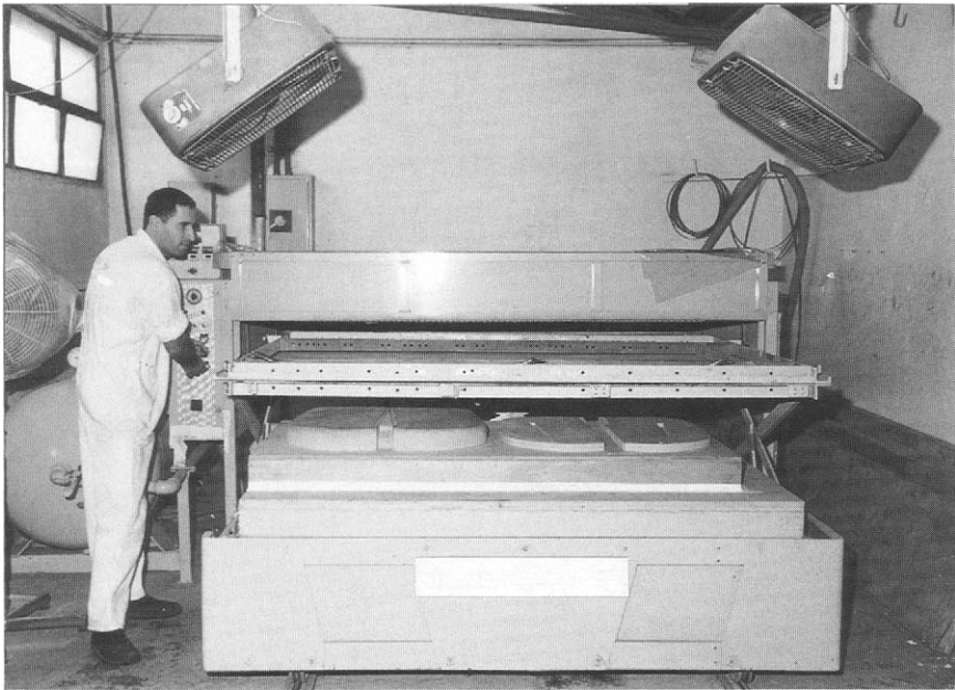
FIG. 9. Vacuum forming in the composite structure shop: A softened plastic sheet takes the shape of a wooden model under vacuum.
