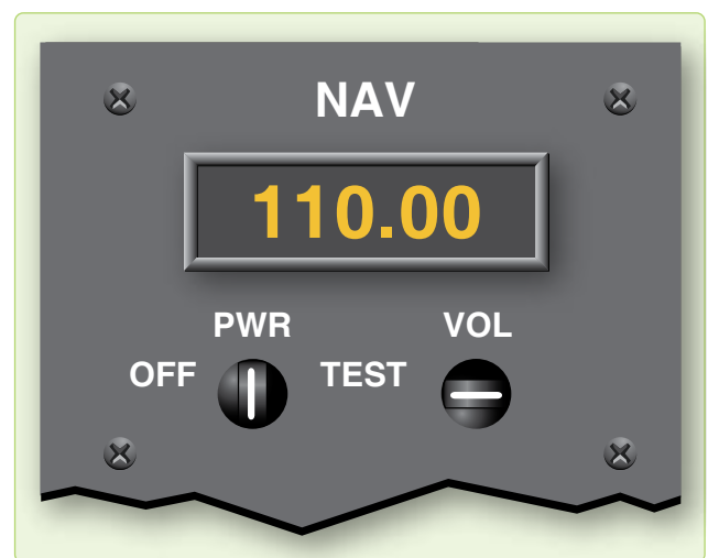
Figure 5-7. VOR navigation control panel.
