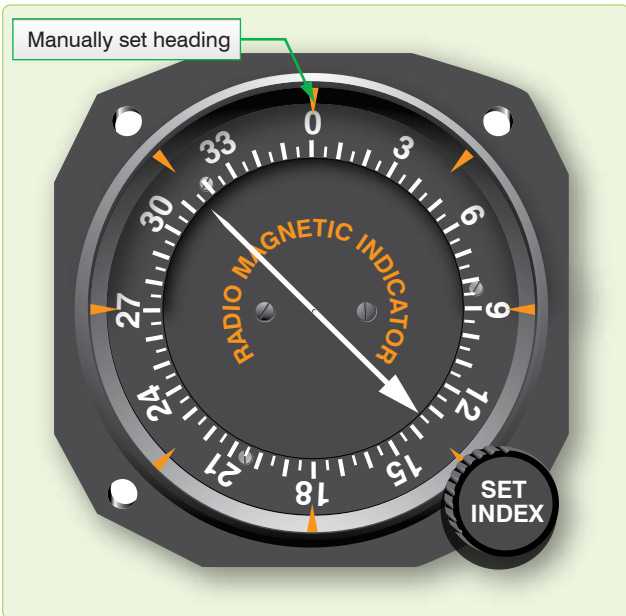
Figure 5-9. Radio magnetic indicator.
