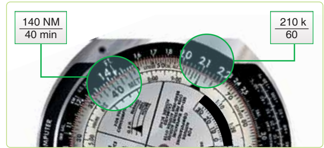
Figure 4-18. Solving for speed when time and distance are known.
