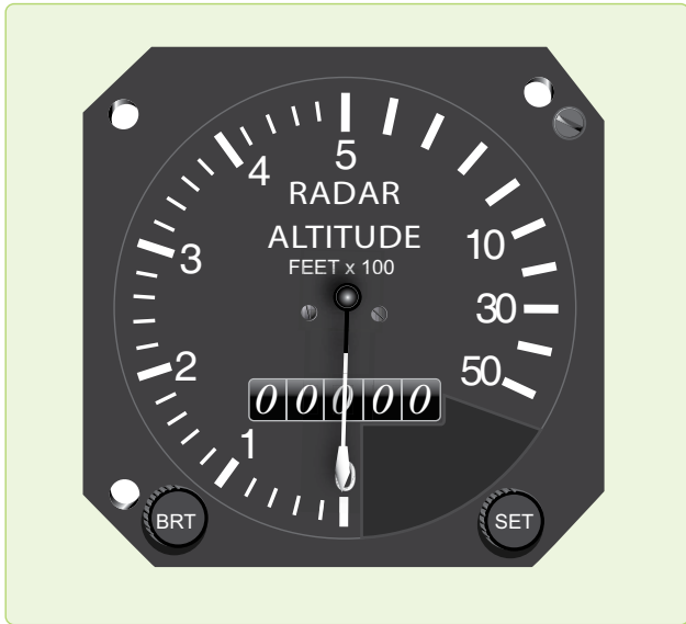
Figure 3-19. High-level radar altimeter.
