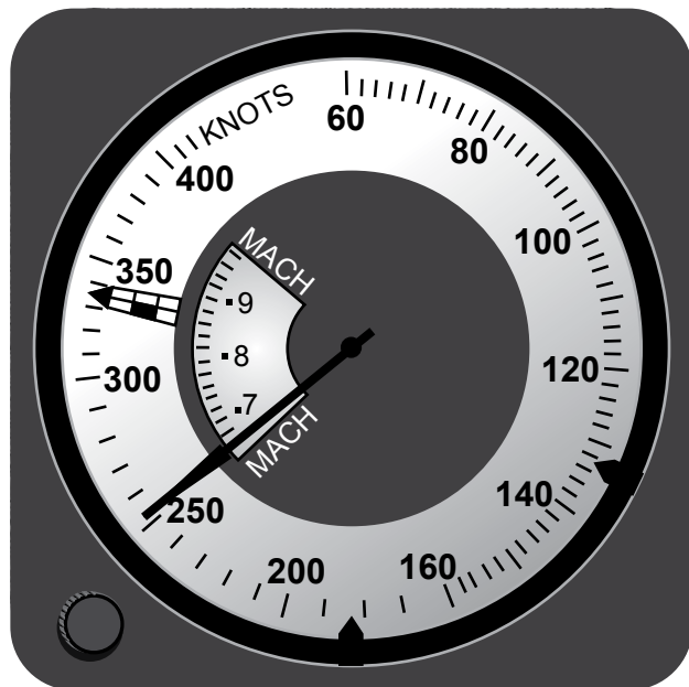
Figure 3-25. Combined airspeed Mach indicator.
