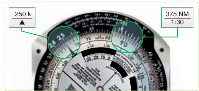
Figure 4-17. Solving for speed when time and distance are known.
