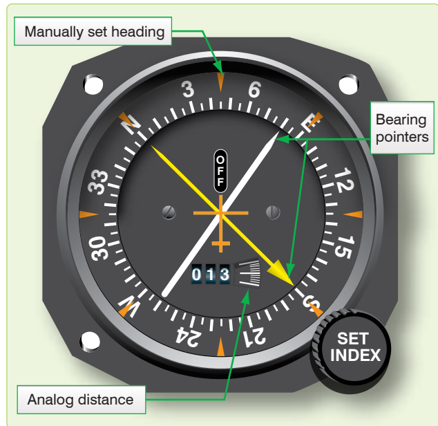
Figure 5-10. Bearing distance heading indicator.
