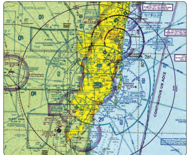
Figure 5-32. Temporary flight restriction (TFR).
