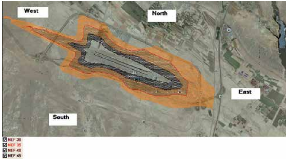
Figure 1. Contours of the noise around the airport. Invert the output of software to decibels: Black contour: 80 dB; Brown contour: 75 dB; red contour: 70 dB; and at last contour 65 dB.
