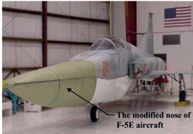
Figure 3. The F-5E aircraft modified by Northrop Grumman [23].
