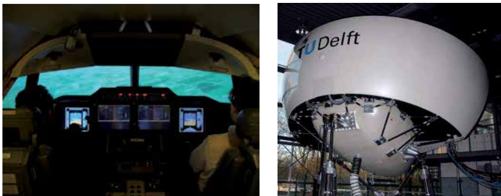
Fig. 12. Evaluation of GARTEUR FM-AG(16) FTFC techniques in the Delft University SIMONA Research Simulator based on reconstructed accident scenarios (Left: Boeing 747 cockpit configuration. Right: visual system dome)
