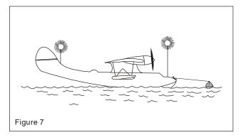
c) If 50 m or more in span a steady white light on each side (Figures 8 and 9) to indicate the maximum span and visible, so far as practicable, all around the horizon at a distance of at least 1.9 km (1 NM).
