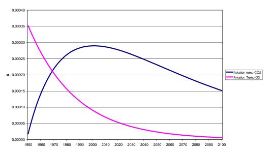
Temperature response from a 'fleet pulse' emission (100 Tg C, EINO<sub>x</sub>=12)
