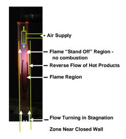
Figure 8: A photograph of a quartz SPRF combustor in operation
