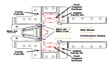
Figure 7: TVC cross section<sup>17</sup>
