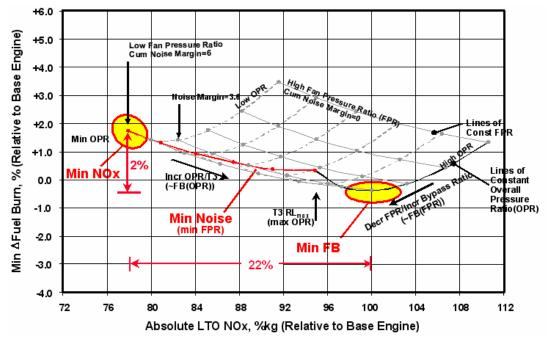
Figure 12: Engine/Airframe Cycle Tradeoffs - Fuel Burn/NOx/Noise Carpet Plot Example
