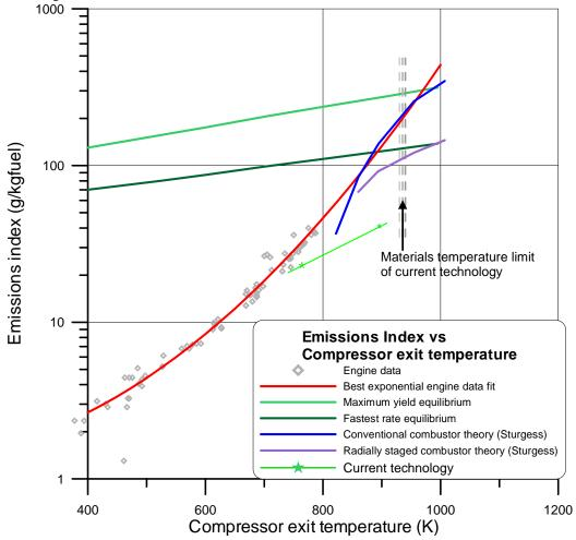
Figure 6: NOx as a function of Combustor Air Entry Temperature
