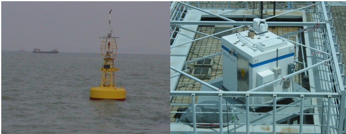
Figure A4-8. Wind shear detection facilities implemented in the early 2000s — weather buoy (left) and LIDAR (right)
