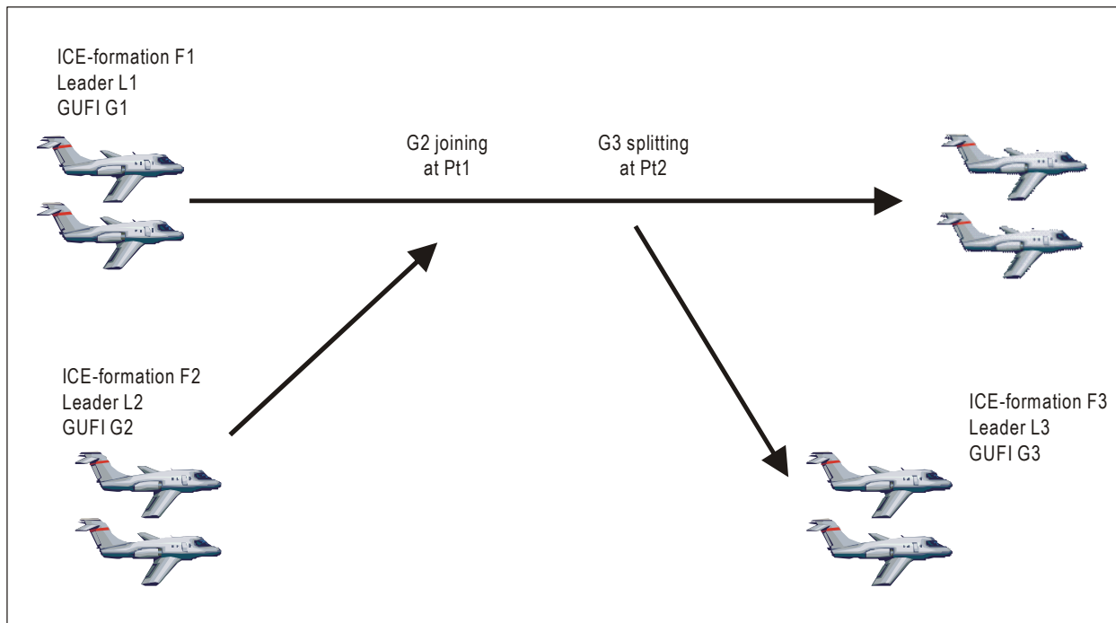
Figure 3-9. Illustration of formations joining and splitting from a main formation F1
