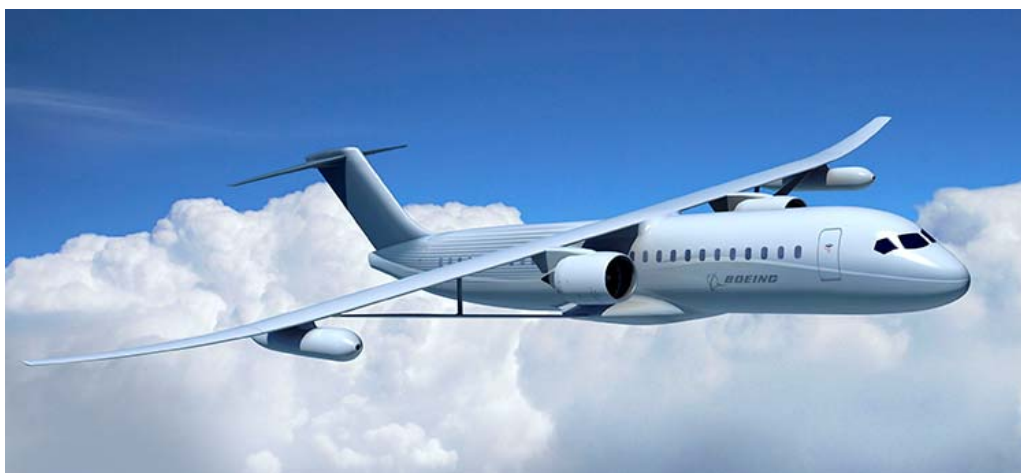
Figure 9-3. TTBW technology aircraft from NASA/Boeing N+3 SUGAR
