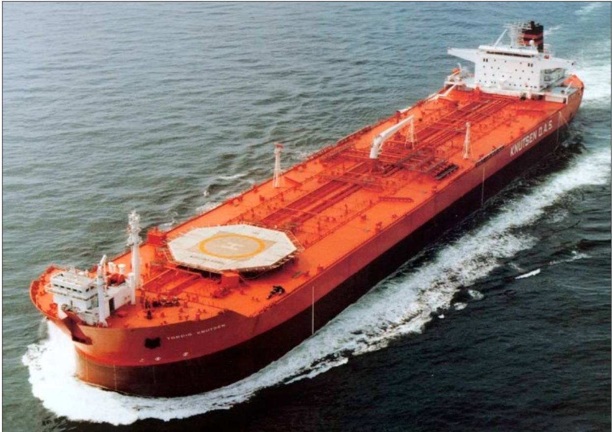
Figure I-1-5. A tanker with a purpose-built mid-ship centreline shipboard heliport
