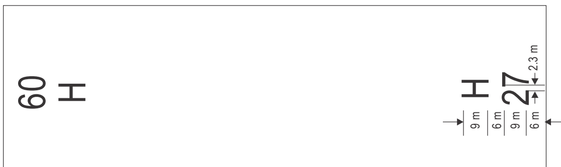
Figure II-5-11. Designation markings for runway-type FATO
