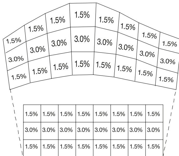
Figure 4-23 – Adjusting a probability map for drift motion when drift forces vary from one place to another in the possibility area (drift distance and area expansion exaggerated for clarity)
