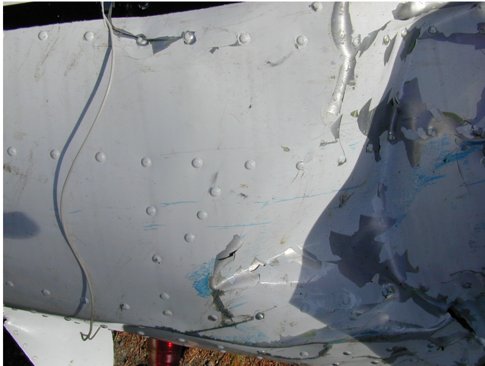
Figure III-10-4. A vertical surface of a fuselage photographed from the side. Note the straight scratch marks and the relatively small angle formed with the longitudinal axis, showing little relative vertical movement in this collision.
