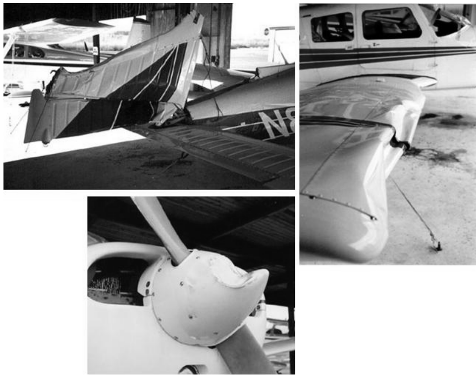
Figure III-9-24 The ductility of metal structures provides macrostructurally visible information regarding an accident.
