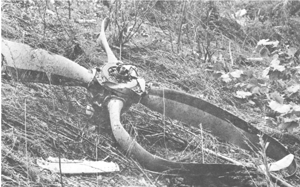
Figure III-12-31. Metal propeller under power at impact
