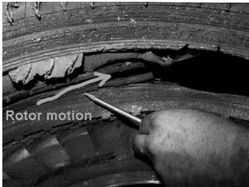
Figure III-12-13. Squeeze-rupture penetration hole
