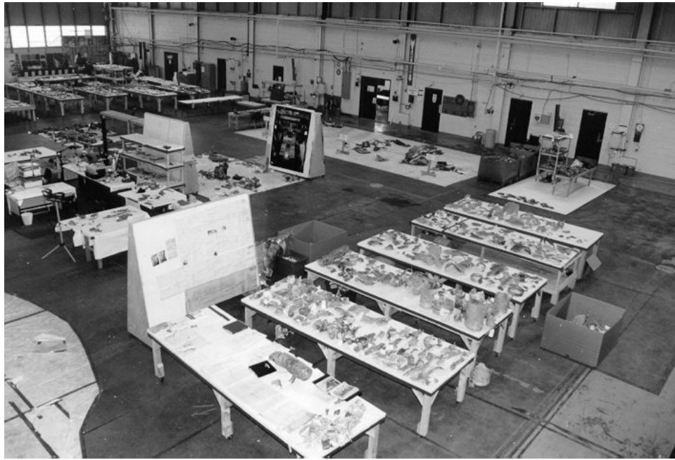
Figure III-8-3. Systems Reconstruction Layout of Swissair 111 (Courtesy of Transportation Safety Board of Canada)
