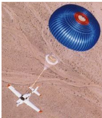
Figure III-13-11. Rocket-deployed emergency parachute system
