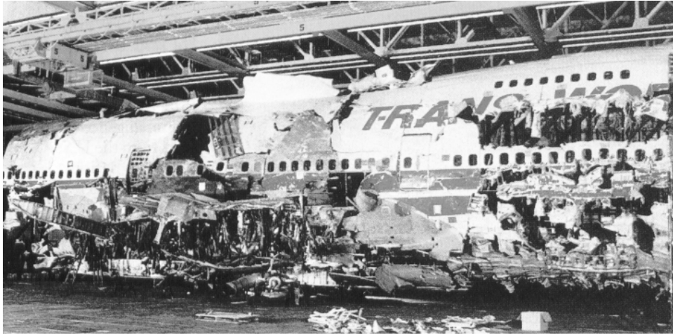
Figure III-8-5. Reconstruction of TWA 800 main fuselage section (Courtesy of U.S. National Transportation Safety Board)
