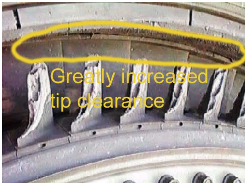
Figure III-12-24. Increased tip clearance caused by overheating
