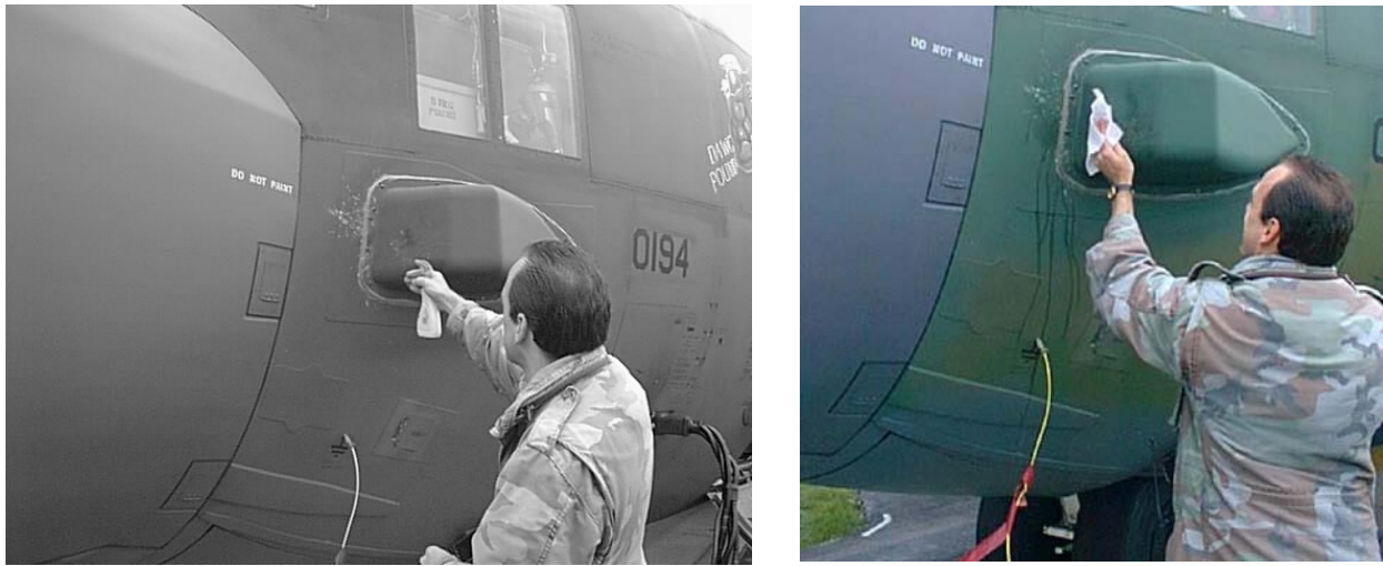
Figure III-5-5. An investigator sprays a suspect area with clean water. He then wipes the area with a clean rag.
