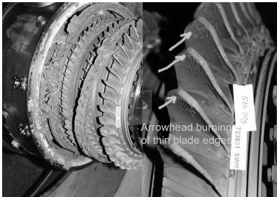
Figure III-12-26. Titanium fire damage (note arrowhead effect)
