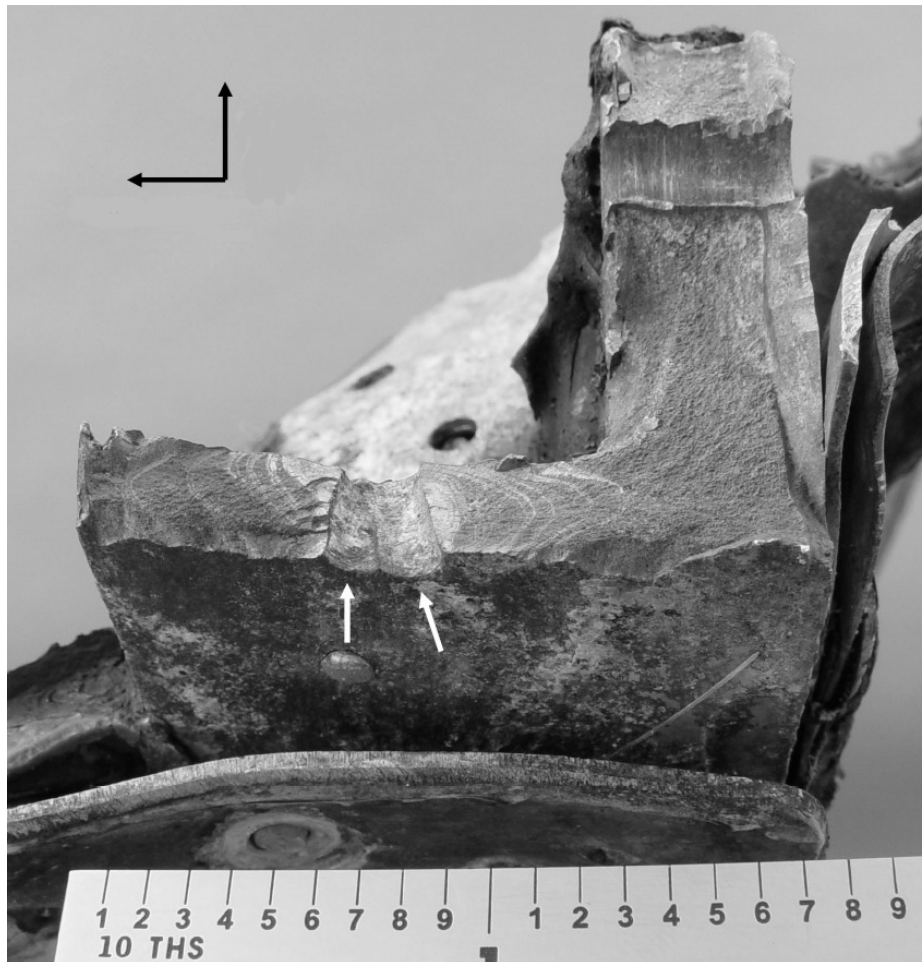
Figure III-9-25. Indications of fatigue cracking in the lower right wing spar cap of the Chalks Ocean Airways Grumman Mallard G73 that crashed in December 2005. This is an example of using accumulated knowledge and experience with metallic structures to identify possible factors in an accident.
