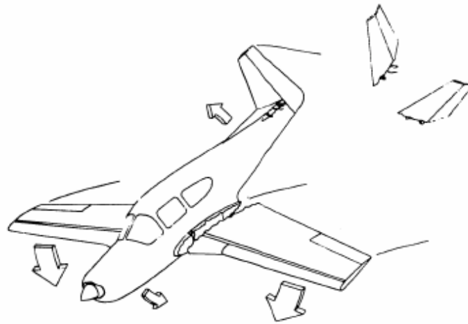
Figure III-9-20. The excessive down load on the wings causes one (or both) wings to fail by down bending.
