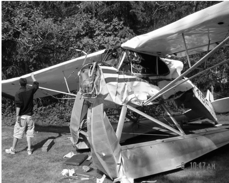
Figure III-5-1. Water impact damage
