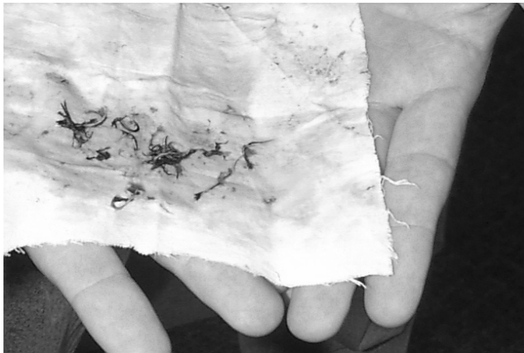
Figure III-5-6. Bird evidence wiped from the aircraft
