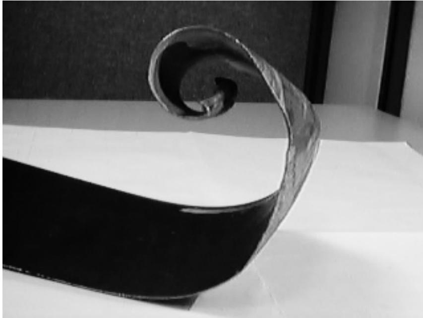
Figure III-12-35. Propeller tip bent forward as a result of high rpm during a low-angle impact
