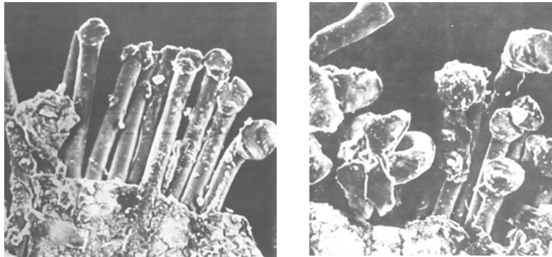
Figure III-19-19. (Left) Controlled-explosion damage to Canadian Nylon 66 sample; (Right) Enlarged view
