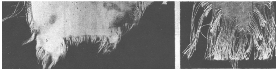
Figure III-9-15. Teasing. Left: Fractured edges "fluffy" due to flapping in airstream. Right: Fracture after tearing.
