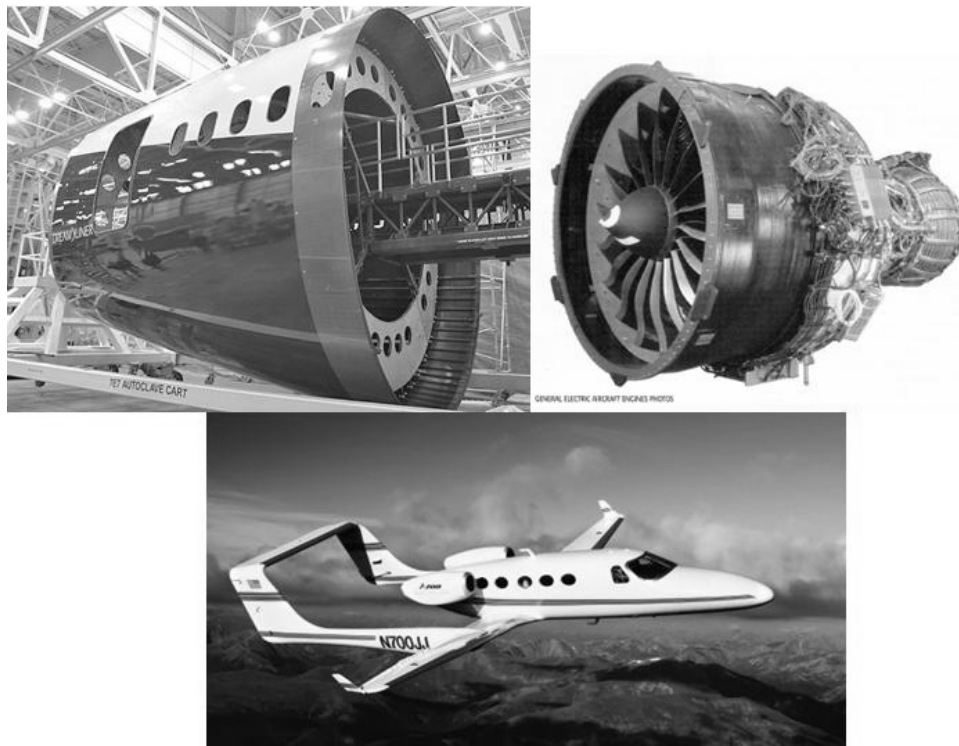
Figure III-9-21. Examples of composite structures (clockwise from top): Boeing 787 fuselage, General Electric GEnx fan blades and case, Adam Aircraft A700 VLJ.
