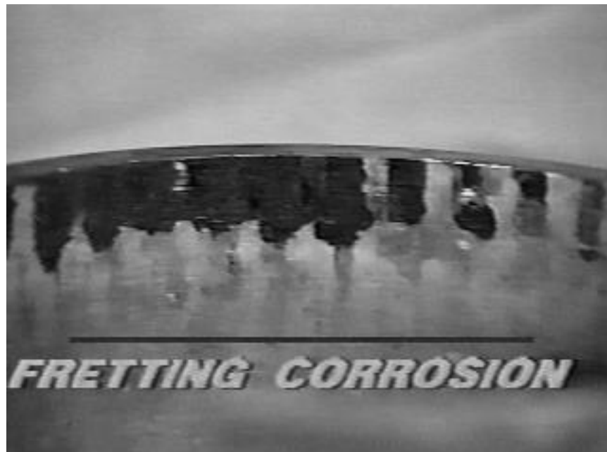
Figure III-9-77. Damage caused by fretting corrosion. Fretting corrosion may be considered as mainly mechanical wear with some combined corrosive action.
