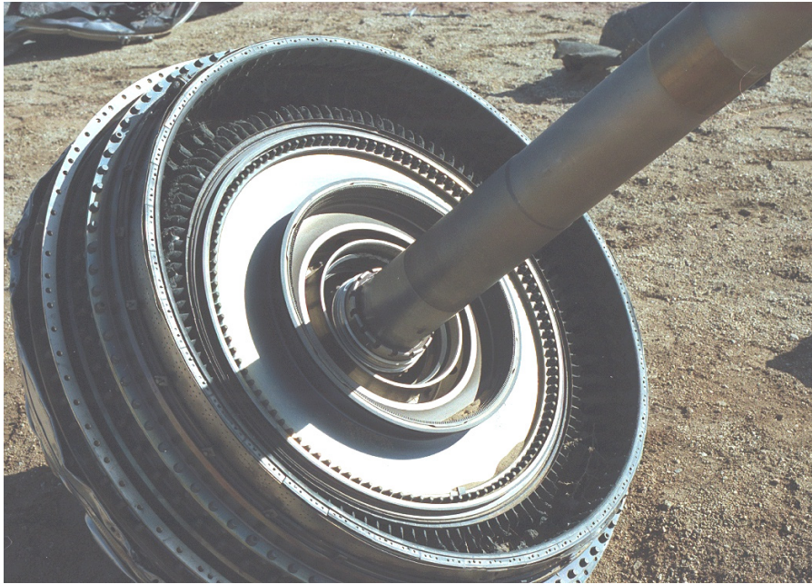
Figure III-2-1. This photograph illustrates the problem of taking photographs on a clear day with bright sunlight as the only illumination. It was made to illustrate heat damage to the turbine section. Note that most of the detail of the damage is lost in the shadows.
