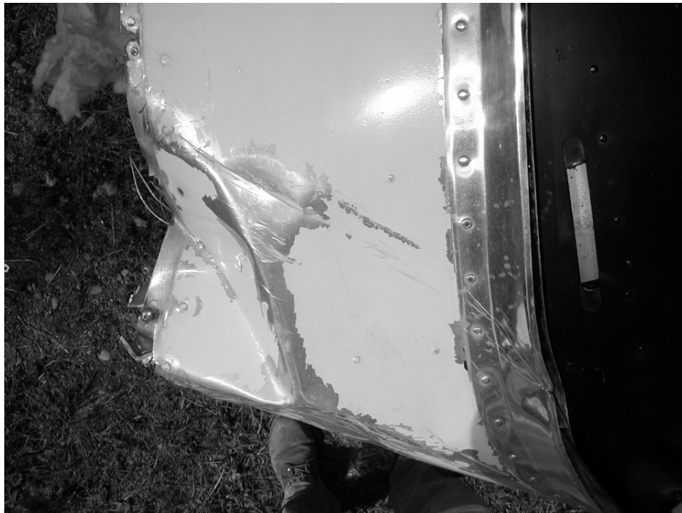
Figure III-10-3. Scratch marks on a horizontal surface photographed from overhead. Note the straight lines.
