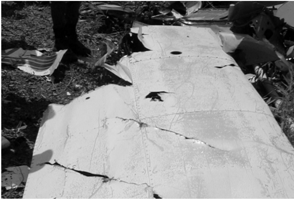
Figure III-10-11. Connecting the mid points of multiple prop slashes will form an equivalent scratch mark.
