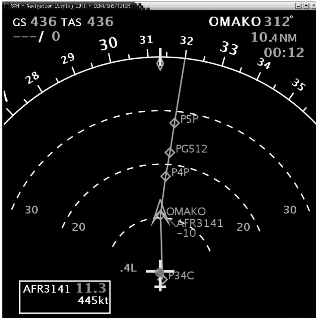
Figure 6-4. Example of a possible future ASA application on an integrated display
