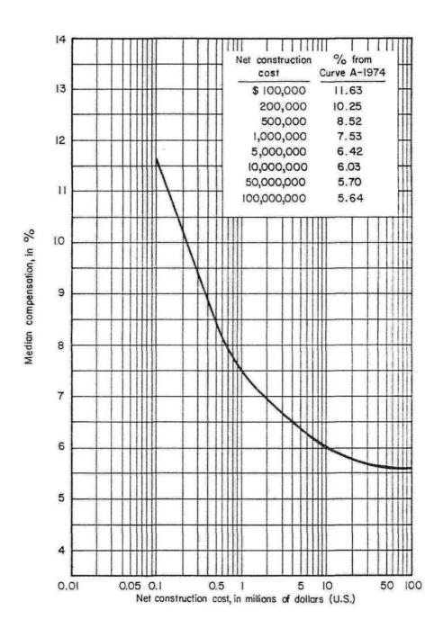
Figure 2-1. Curve A, Median Compensation for Basic Services
