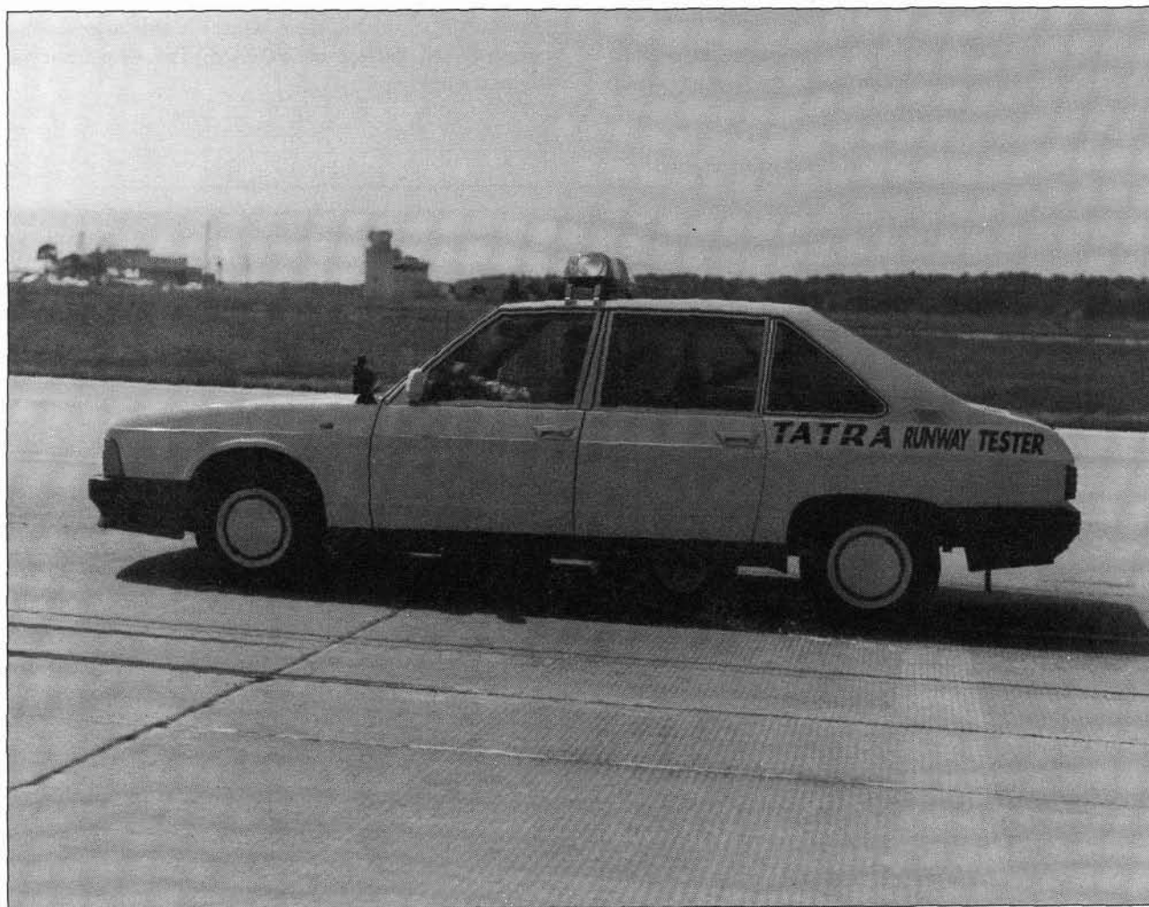
Figure 5-12. Tatra Friction Tester
