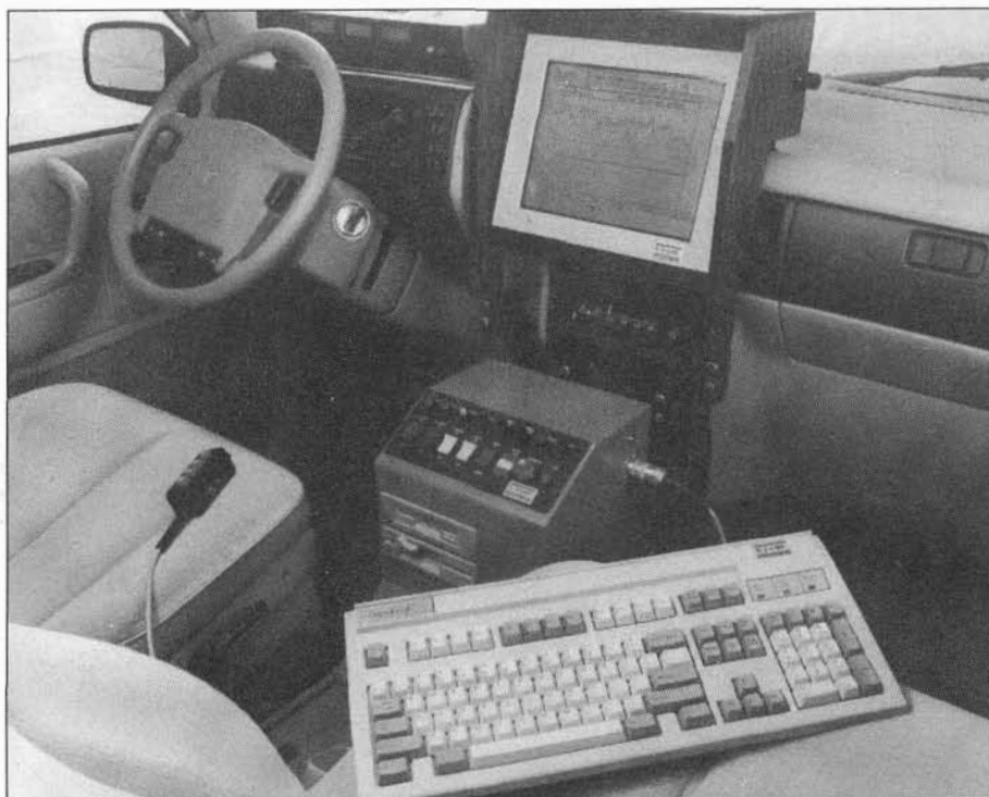
Figure 5-7. The vacuum fluorescent display unit and keyboard for the Runway Friction Tester
