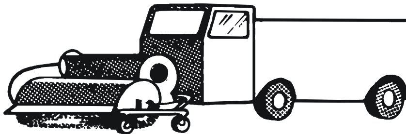
Large swath, heavy duty — over 3.6 m — pushed type with two engines, front blower — conventional cab
