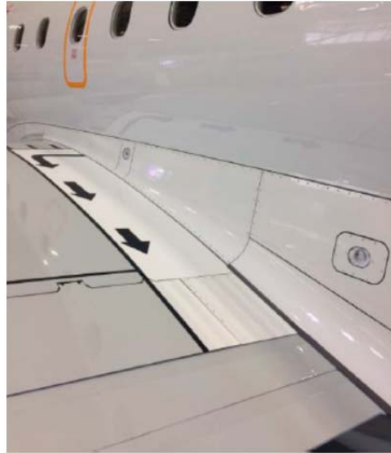
Figure 4-11. Example of over-wing markings (courtesy of Embraer)
