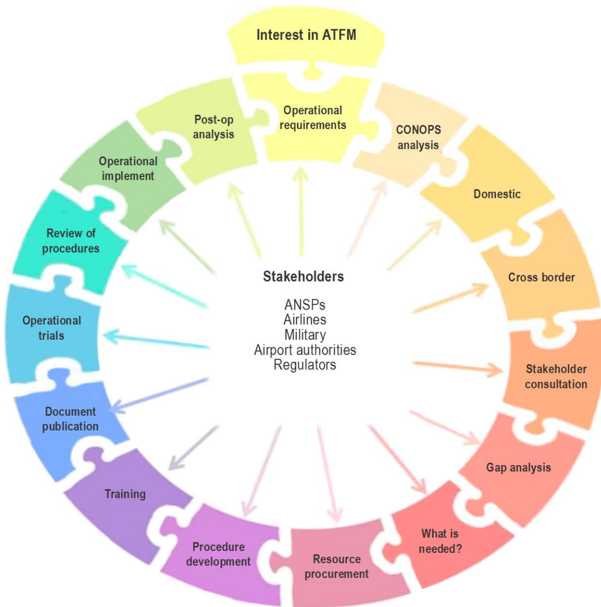
Figure II-8-1. ATFM implementation steps
