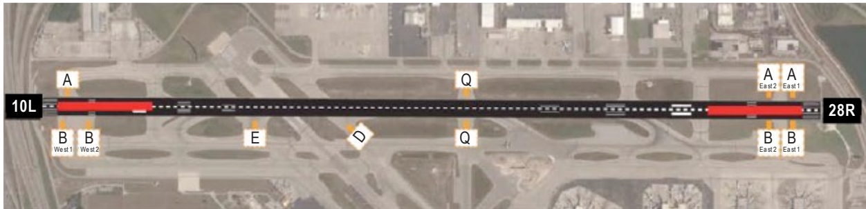
Figure 11-10. RWSL at Fort Lauderdale–Hollywood International Airport (FLL/KFLL) Photo source: FAA
