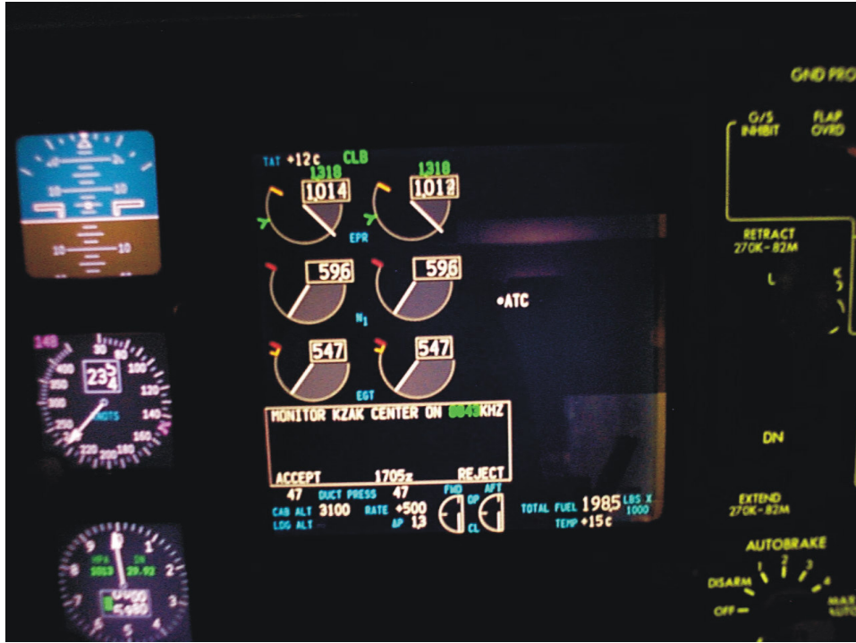
Figure 3-8. Visual indication of an incoming CPDLC message
