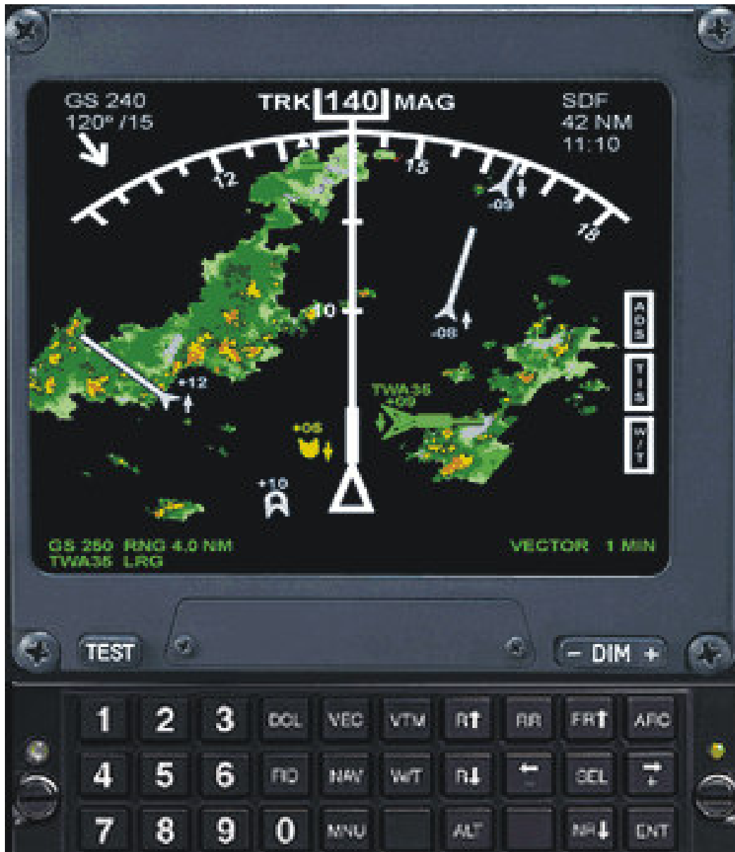
Figure 8-3. Example of a navigation display with an integrated CDTI and weather radar
