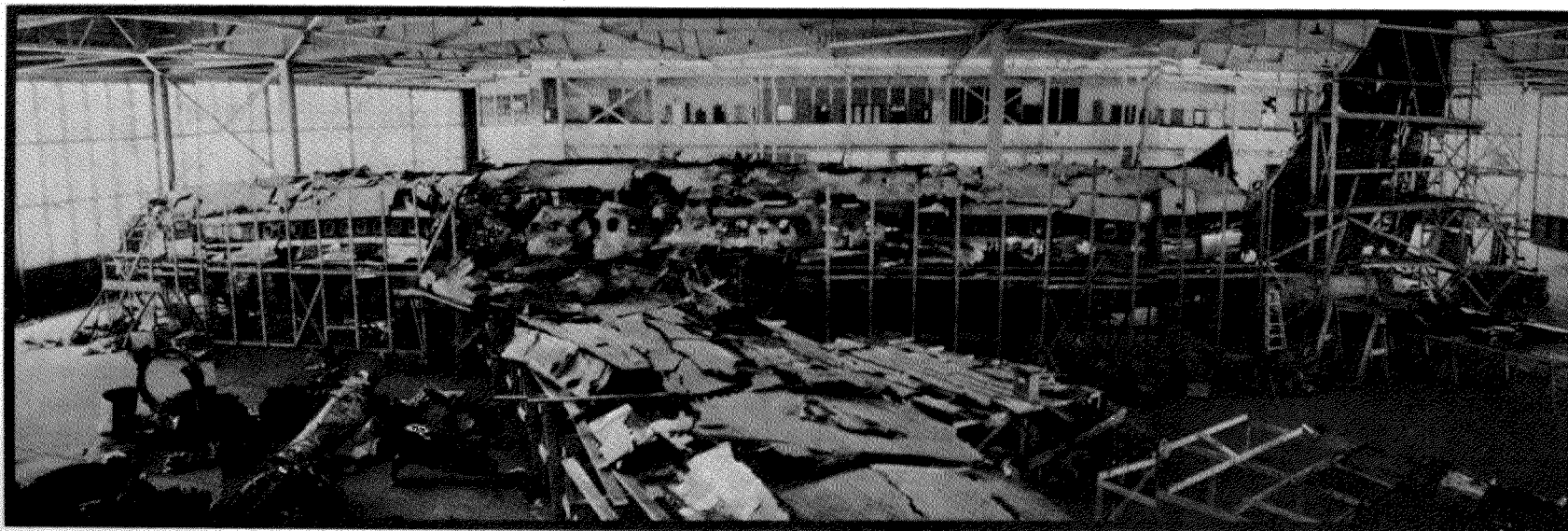
CIVIL AERONAUTICS BOARD WRECKAGE MOCKUP
