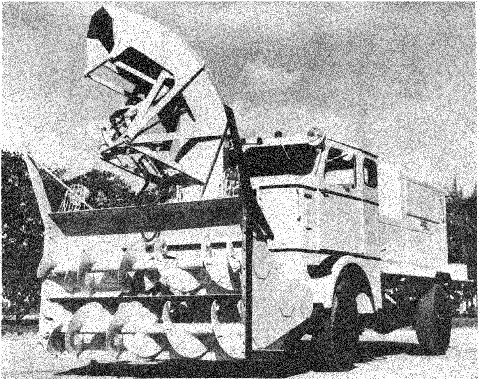
4. Rotary type snow blower showing feed augers and impeller behind the augers.
