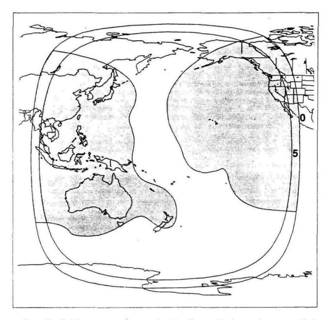
Note. — The shaded areas represent the east and west hemi-beams, while the outer rings represent the Cband (6/4 GHz) and Ku-band (14/12 GHz) global beam coverage at elevation angle contours of  $0^{\circ}$  and  $5^{\circ}$ . The  $0^{\circ}$  elevation angle contour is the theoretical extent of coverage, while the  $5^{\circ}$  elevation angle is considered to be the practical extent of coverage according to nominal design criteria.
