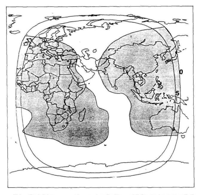
Note.— The shaded areas represent the east and west hemi-beams, while the outer rings represent the Cband (6/4 GHz) and Ku-band (14/12 GHz) global beam coverage at elevation angle contours of  $0^{\circ}$  and  $5^{\circ}$ . The  $0^{\circ}$  elevation angle contour is the theoretical extent of coverage, while the  $5^{\circ}$  elevation angle is considered to be the practical extent of coverage according to nominal design criteria.
