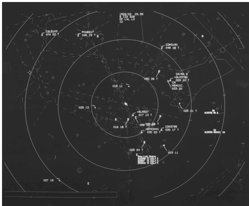
FIGURE 3.2 Sample of data link information at the controller's workstation. The sample shows experimental display of resolution advisory data downlinked from the traffic alert and collision avoidance system (TCAS). Source: Photo courtesy of the MITRE Corporation.
