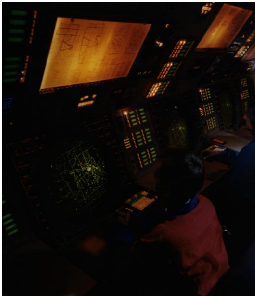
FIGURE 6.4 Center TRACON automation system (CTAS) descent advisor (DA) display. Source: National Aeronautics and Space Administration.
