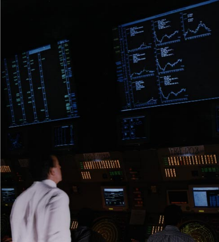
FIGURE 6.3 Center TRACON automation system (CTAS) traffic management advisor (TMA) large screen displays. Source: National Aeronautics and Space Administration.
