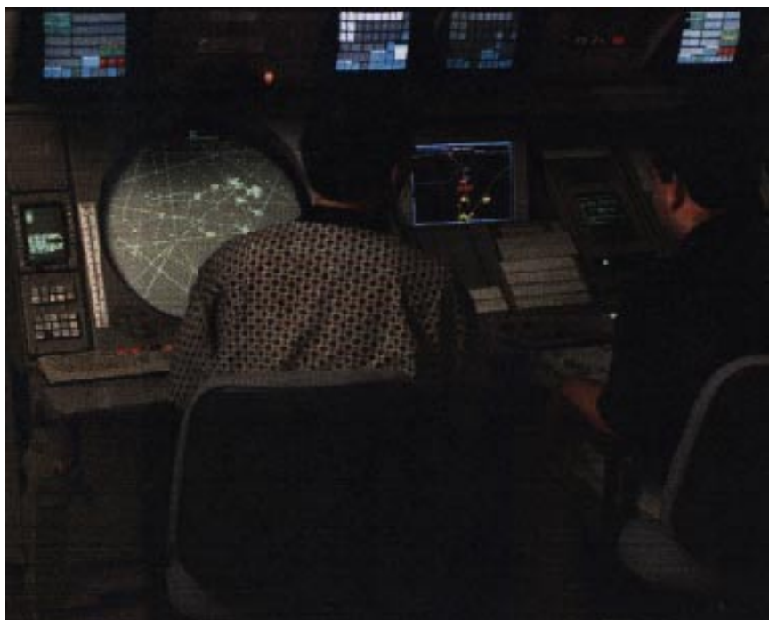
FIGURE 6.8 User request evaluation tool (URET) at controller's workstation. Source: Photo courtesy of the MITRE Corporation.
