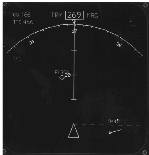
FIGURE 5.1 Sample traffic alert and collision avoidance (TCAS) display, showing a target 19 miles ahead. Source: Photo courtesy of the MITRE Corporation.
