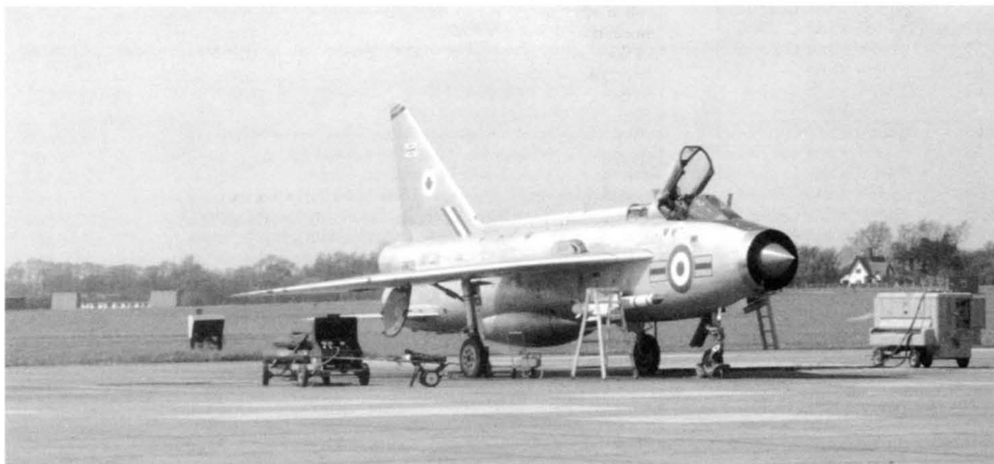
F.1 XM139 of the Wattisham TFF. On top of the wing is one of the ammunition tanks (the F.1 had a pair of 30mm Adens in the cheek positions behind the panel to the rear of the two red triangles, called 'elephant ears'). In the TFF rôle these were not fitted but the tanks were filled with ballast to compensate and maintain the aircraft trim. The black trolley on the left is an oxygen trolley (the F.1 and F.1A had a gaseous oxygen system). The badge on the fin is the later Wattisham TFF badge, a stylized rear view of a cat with its tail raised and its whiskers the horizontal points at the side. This badge was chosen by TFF pilots because that is what they showed the intercepting pilots – their backside! The cat's tail represented the fins and the whiskers, wings and tailplane. A puckered orifice was painted beneath the tail, in place of the No.1 jet pipe (No.1 was left off). Pete Nash
