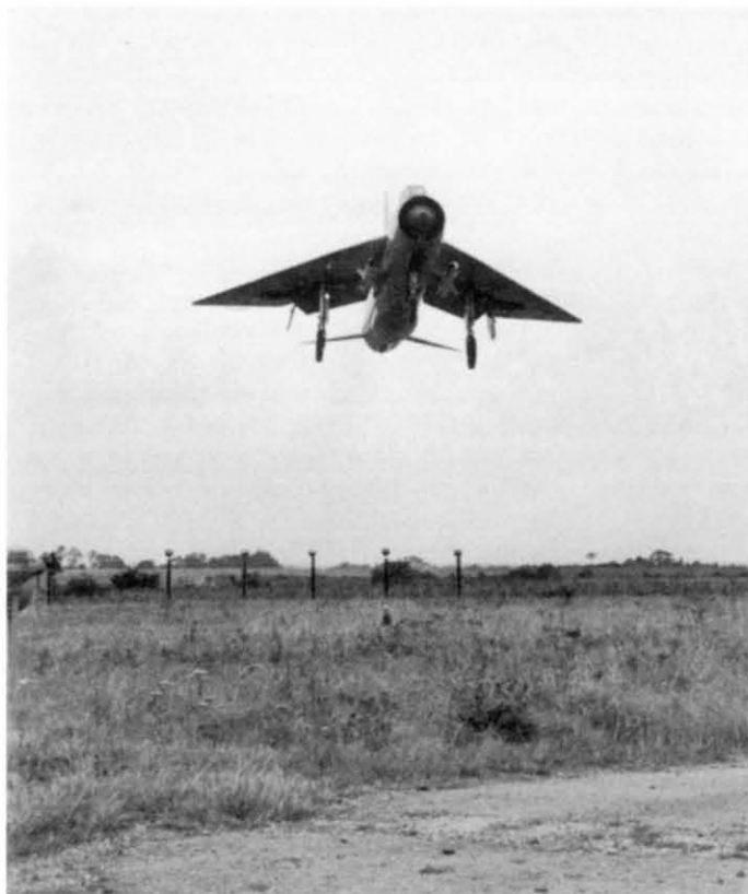
The 'crab' technique was recommended for approach and landing. A sufficiently long final approach should be flown in order to assess the drift. Normal approach speeds were used and drift kicked off as the aircraft was rounded-out; aileron might have to be used to counteract roll if there was much drift to remove. The student had to be initially told to keep the ailerons neutral after touchdown; later, he might be shown the effect of using downwind aileron.
