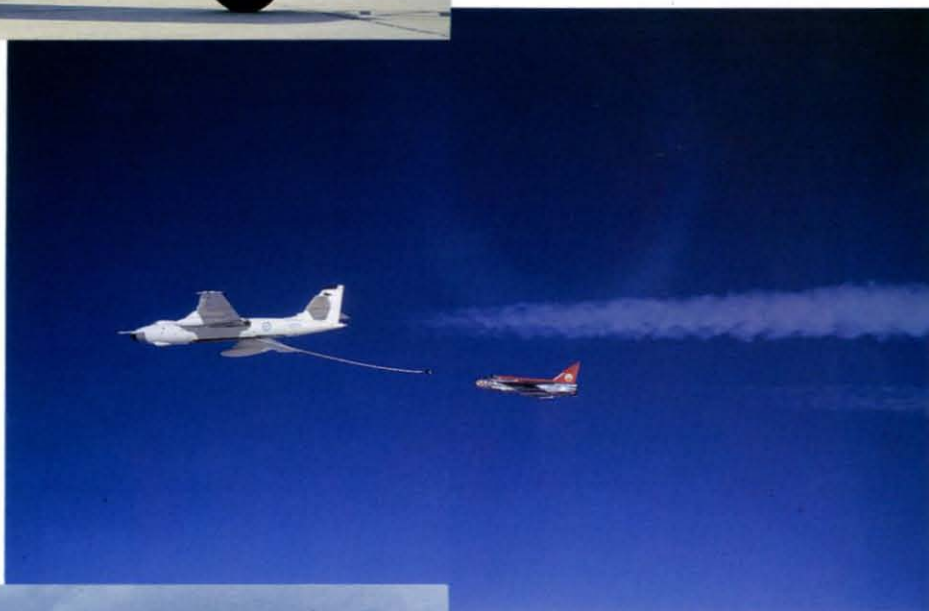
F.1A XM173/C of 56 Firebirds Squadron, one of only twenty-four built, and the first Lightnings to be fitted with a production in-flight refuelling probe, closes in to refuel to tank from Vickers Valiant XD814, January 1964. In 1965 the Valiants were scrapped following metal fatigue problems. Brian Allchin
