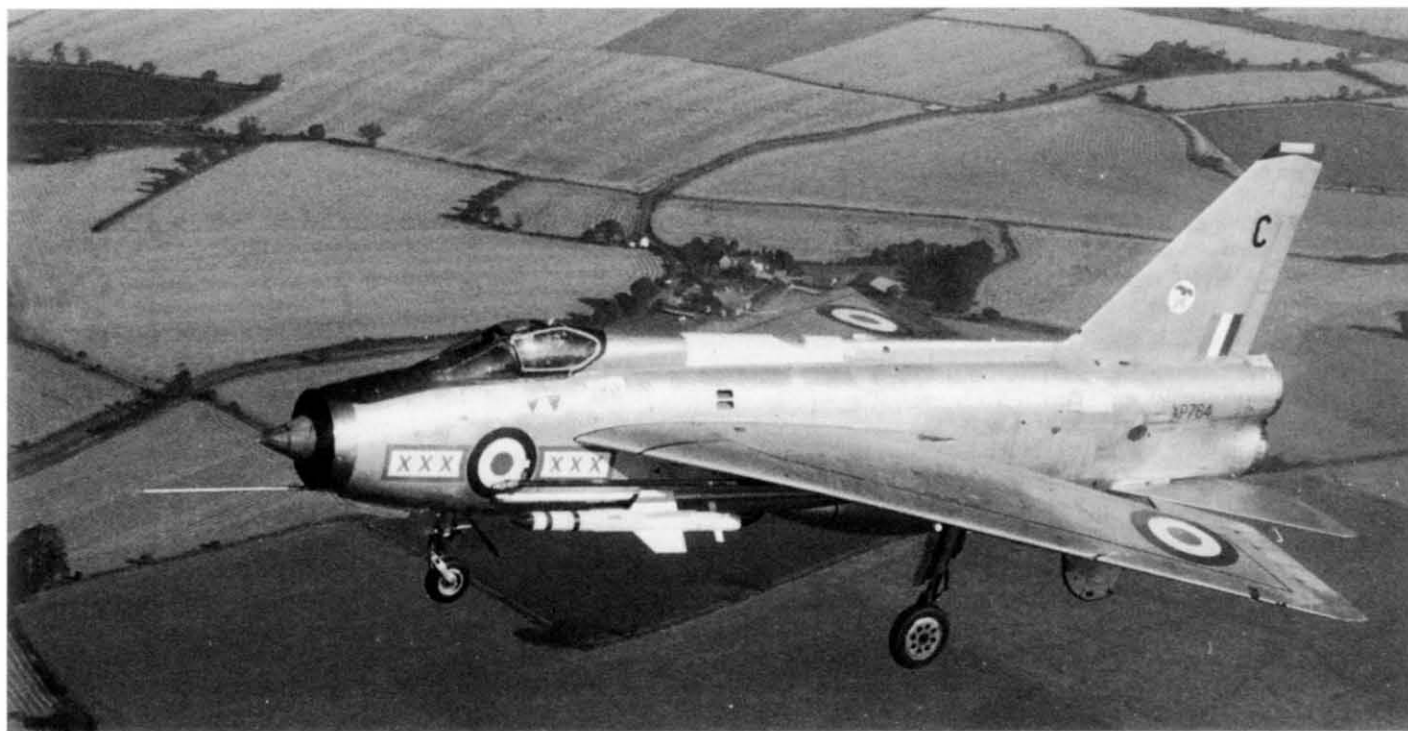
Circuit work commenced right at the beginning of the conversion. The flapless circuit was practised in order to demonstrate to the student the approach pattern in the event of a landing without the use of flaps or airbrakes. The systems failure was assumed from the over-shoot from a normal circuit and the student was required to perform the complete circuit with the flaps and airbrakes inoperative. It was strongly emphasized to the student that if he had to overshoot with a known failure of this nature, he must not raise the undercarriage. Dick Bell
