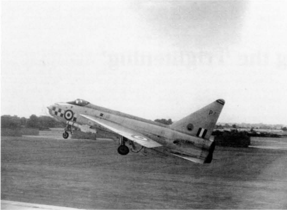
F.1A XM182 of 56 Squadron using cold power for take-off from RAF Wattisham in July 1961. The Lightning's acceleration on take-off was spectacular, even without re-heat. The E-Type Jaguar, then the epitome of sports cars, was out-accelerated to 60mph by a factor of about three – and the Lightning could reach 500mph in just over forty seconds . . . its pilots were indeed privileged men. Aeroplane
