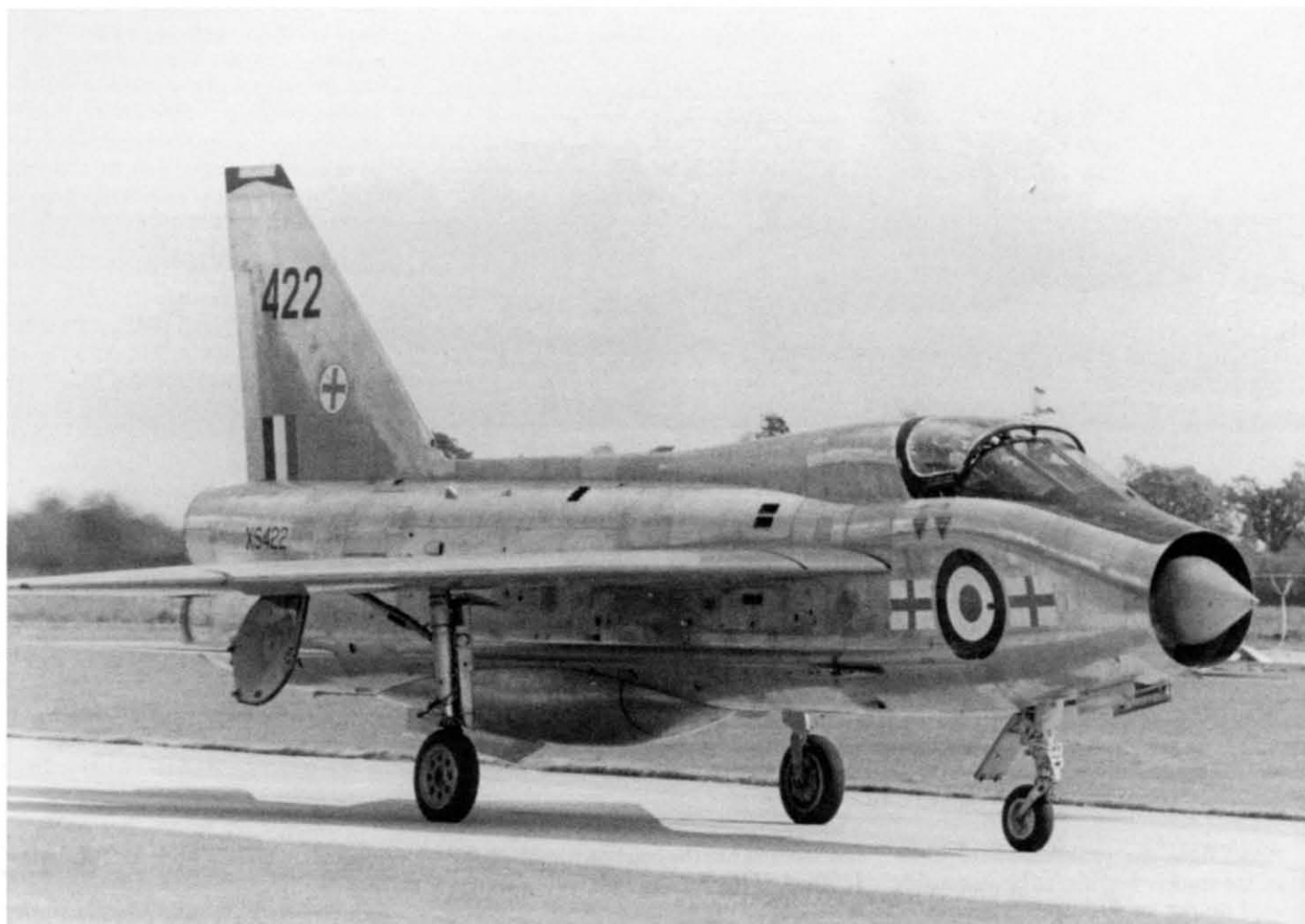
Once clear of the runway, and with No.1 engine below ten per cent power, flaps and airbrakes would be selected 'in' and all the non-essential switches turned 'off'. It was important to check the recovery of the services hydraulic pressure, thus ensuring that both pumps had been checked. Ronald Johnson
