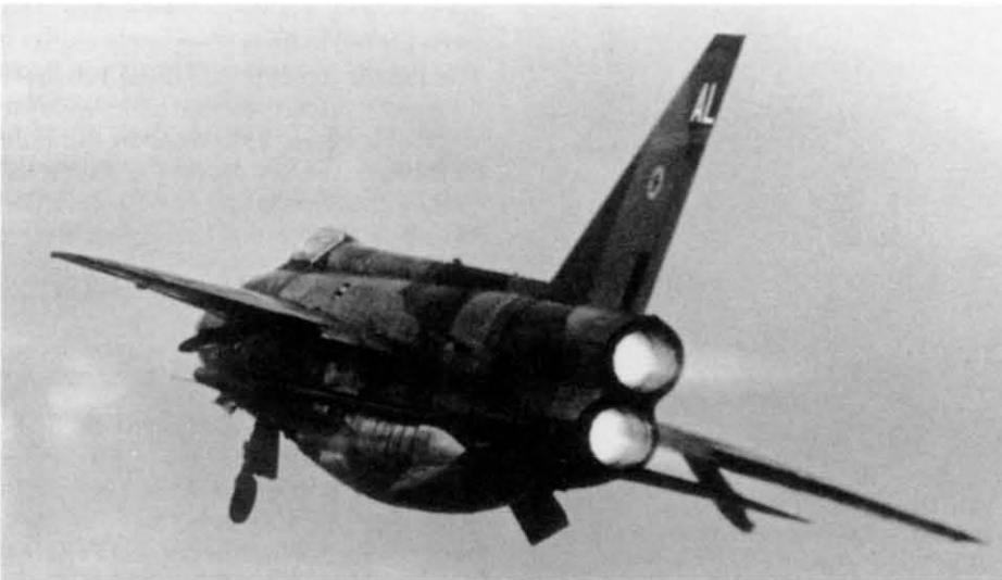
Once airborne with the undercarriage selected and locked up, and at a safe climbing attitude, a turn onto the climbing heading could begin. When the speed reached 420kt, the angle of climb was then increased to eighteen degrees to maintain 450kt. Ken Johnson
