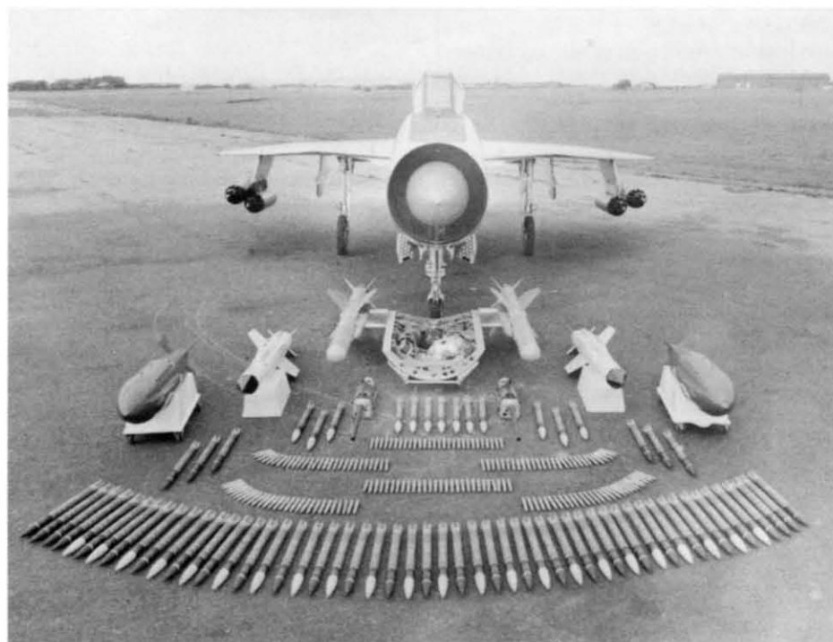
The formidable weapons load options available to the F.53. Two Firestreak or two Red Top, plus two 30mm Aden cannon with 130 rounds each (housed in the forward section of the ventral tank), forty-eight 2in (51mm) spin-stabilized rockets in the fuselage forward weapon bay in place of missile pack and two 1,000lb (450kg) HE bombs. The rockets are housed within the fuselage in twin retractable launchers that automatically extended outwards and downwards in one second for firing and closed again after attack. The rockets were designed to fire with optimum dispersion for hitting the target. They fired in 'ripple' salvos whereby two were fired automatically every twenty-five milliseconds. Single 'ripple' salvos could be fired from first one and then the other launcher, or twin 'ripple' salvos could be fired from both launchers simultaneously. Each Matra Type 155 launcher (two proposed twins shown here) could carry eighteen 84mm SNEB 13½lb (6kg) rockets. BAC
