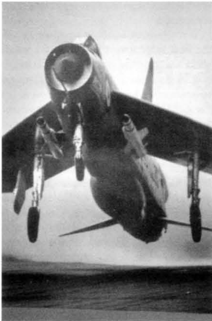
Due to the high fuel consumption when re-heat was used and the consequent reduction in total endurance, only one dual and one solo re-heat take-off and climb were carried out during OCU training. Fuel used on a re-heat climb only exceeded that used in a cold climb by a small margin. Distance to height was 28nm on cold power, and 16nm on re-heat; while time to height was 3fl minutes on cold power and 2fi minutes on re-heat. via Bruce Hopkins/Aeroplane
