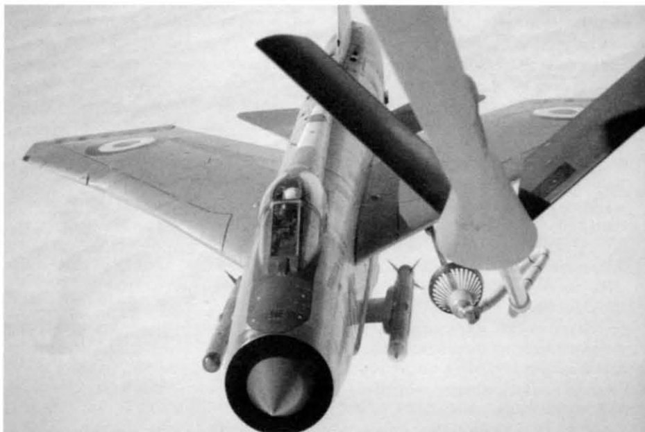
The loss of the Valiant force in 1965 left the RAF with no tanking facilities so the USAF made available three KC-135s over a six- to nine-month period for much-needed in-flight refuelling practice. Operation Billy Boy , as it was called, began on 5 April 1965, with 1fi hour sorties with 23 and 74 Squadron's Lightnings, refuelling with 3,000lb (1,700kg) each sortie. The KC-135's rigid refuelling boom to which was attached a 7ft flexible hose-and-drogue called for a much different receiver technique to that used on the hose and reel-equipped Valiant Brian Allchin
