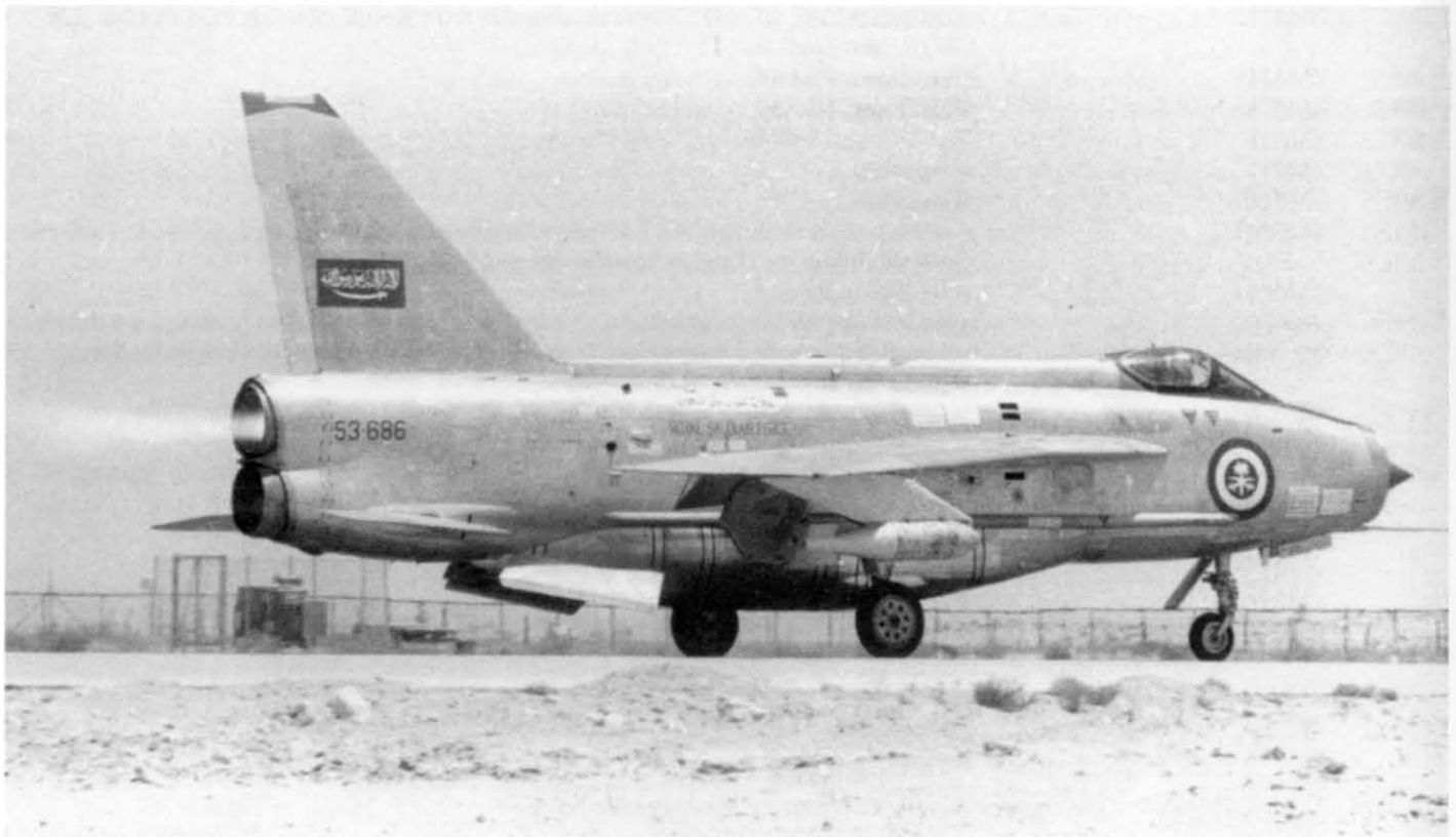
F.53 53-686 of the Royal Saudi Air Force rolling on take-off with re-heat lit and carrying 1,000lb (450kg) practice bombs. Aeroplane
