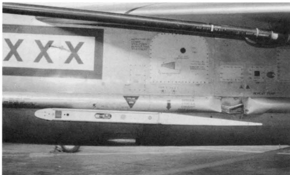
Damage to XP755/E of 29 Squadron after the loss of its drill round missile in flight in June 1972. Note also the skin tear between the last two Xs on the Squadron insignia. The slightly misaligned rear part of the launch shoe is the ammonia bottle. At the front can be seen the flush contact pads supplying electrical current to the missile, while air and ammonia is supplied through the oval aperture. Just discernible on the pack below the electrical connectors is a vertically aligned safety panel with a quick release toggle. The missile safety breaks were placed here whenever the aircraft was carrying live missiles, so that if it landed at another airfield then the missiles could be made safe. The same idea was used on Red Tops, but using different plugs. Pete Nash
