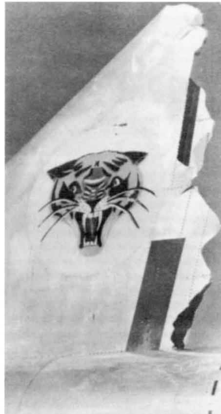
The tail of 'Finless Jim' Burn's aircraft, XM142, after he successfully landed it following the loss of its rudder and a considerable proportion of the fin. via Mike Harris
