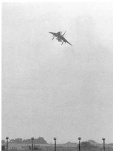
The turn onto the final approach would start at about one runway's length from the end of the runway. If the wind was down the runway, approximately thirty-five degrees of bank would be sufficient, and a rate of descent of about 1,000ft (300m)/minute would be aimed for. Dick Bell Collection
