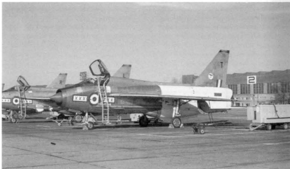
A continuing problem with the Lightning was fuel and hydraulic fires. The two engines mounted above each other, No 1 below, and No 2 above and behind, both had long jet pipes close to the external skin. In an attempt to solve some of the in-flight fire problems 29 Squadron's XS459/T was loaned to BAC in the spring of 1972 for trials, though it remained on the squadron. The safety equipment was removed from the right-hand seat and small reservoirs of blue dye were placed in strategic places around the airframe. A control box operated by the BAC test pilot took the place of the safety equipment and the fuselage was painted with white distemper so that the dye trails could clearly be seen. XS459 is now on display at Wellesley Aviation at Narborough, Norfolk. Pete Nash
