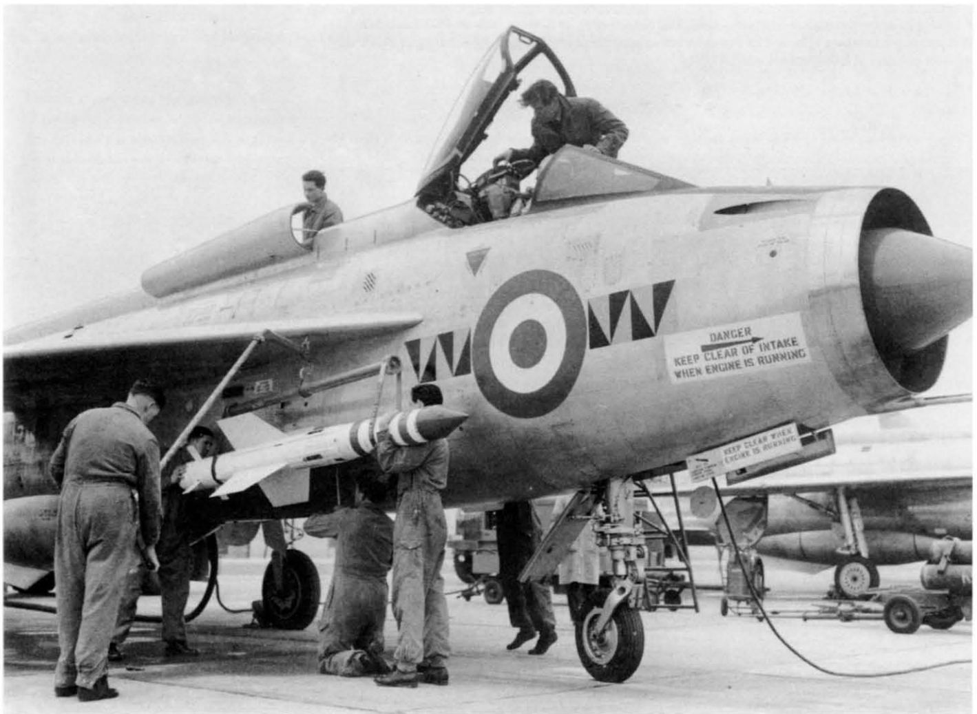
Ground crew hoist a Firestreak missile into place on the side of a F.1 of 74 Squadron at RAF Coltishall in 1961. It usually took between seven and eight minutes to refuel and rearm, from wheel stop to engines start. The pylons on which the missiles were carried contained ejector chargers so that they could be jettisoned in an emergency. via EDP
