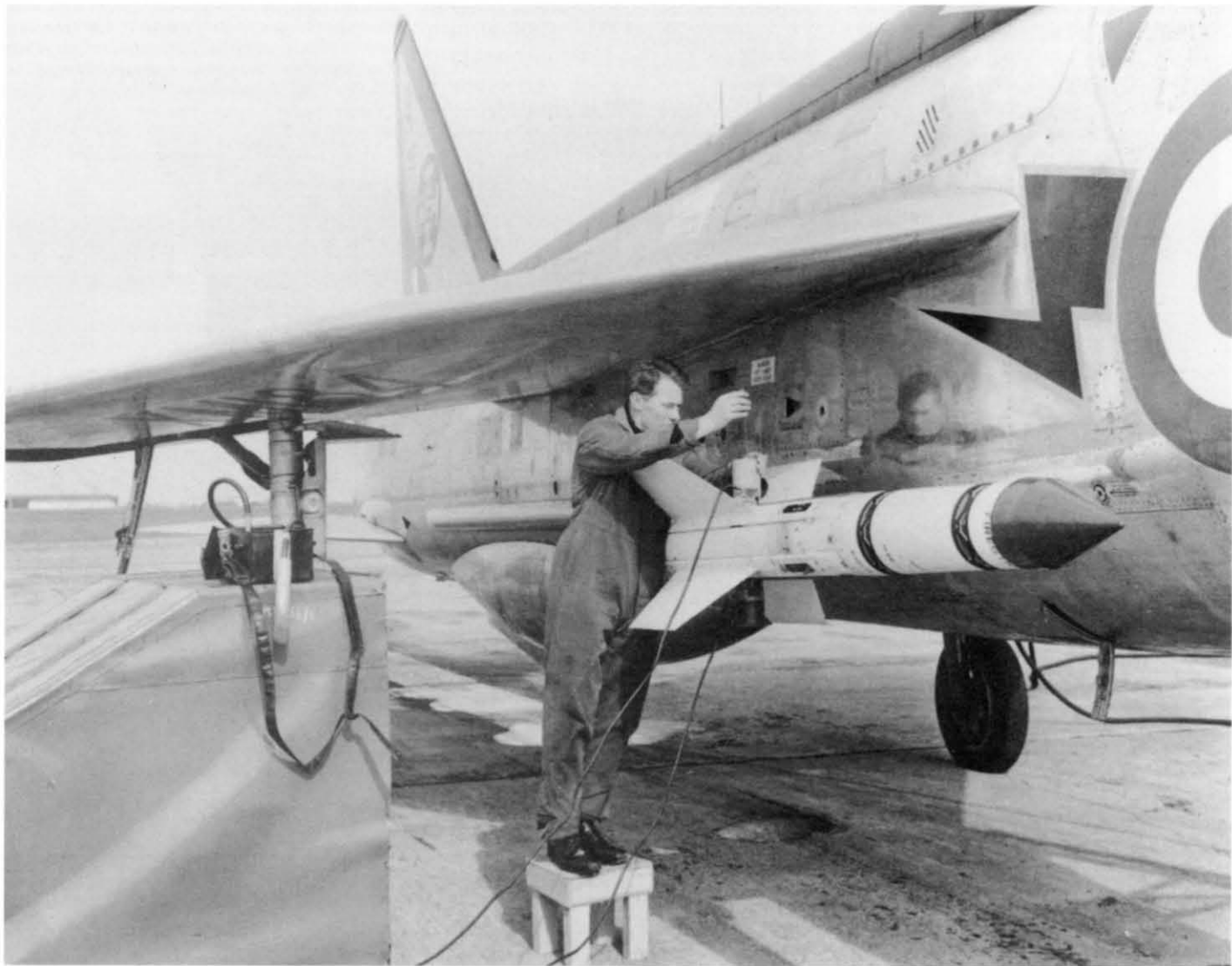
Final preparations and testing of Firestreak missile prior to firing at the missile practice camp, RAF Valley, in March 1964. The aircraft is Lightning F.1A XM184 'A'. George Black
