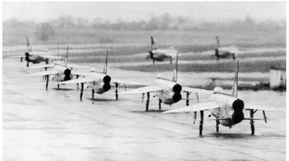
The Firebirds taxi out at Wattisham, each staggered left and right to avoid the jet efflux of the aircraft directly in front. via Dave Seward
