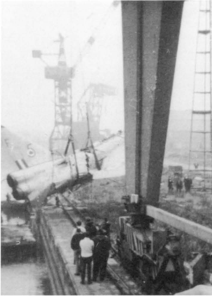
F.6 XS894, which crashed into the sea off Flamborough Head on 8 September 1970, is lifted ashore (for movement to RAF Binbrook) from the bows of the recovery vessel Kinless after recovery from the sea bed. The air brakes are extended, indicating that the pilot, Major Bill Schaffner, was flying very slowly when he hit the sea. Jonathan Falconer
