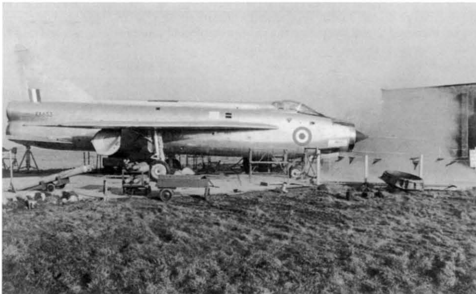
XA853, the second of three P.1B prototypes, was used for gun trials and is seen here at the firing-in butts. Pilots in the AFDS discovered that gun firing in a Lightning was not as successful as missile firing and they proved that the pilot attack gunsight was very basic and not so good under g conditions using lots of angle. However, guns were a very useful weapon to have and almost all pilots mourned their passing in the F.3 which was introduced in 1962. Guns were only reinstated in 1970 when it was decided to fit two Aden cannon into the front of the ventral tank of the F.6s. via Pete Nash
