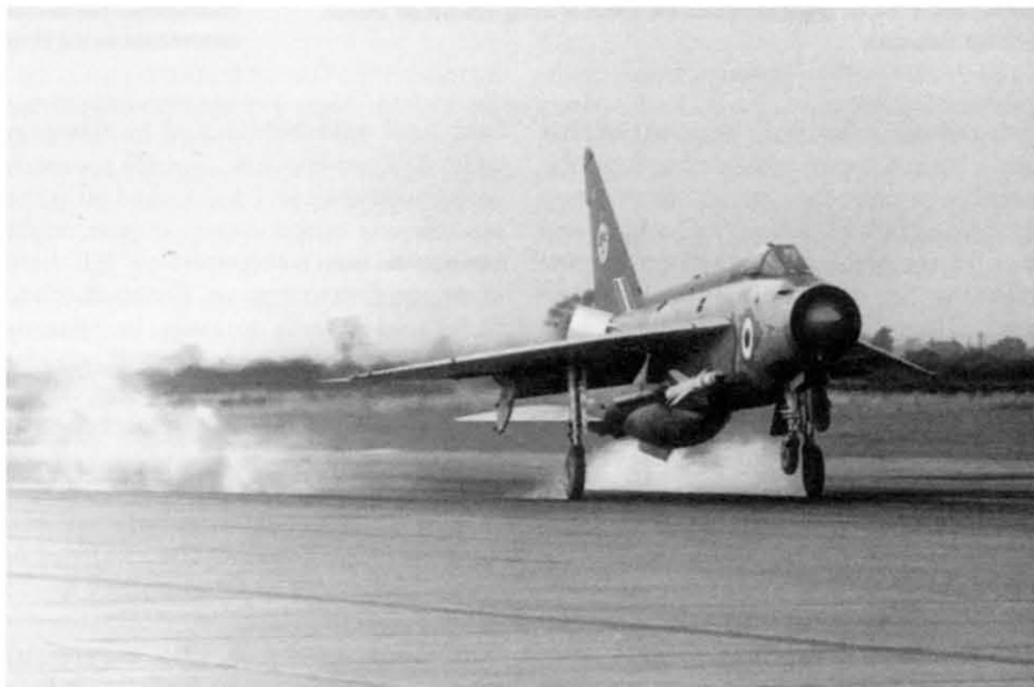
Touch-down speed would be about 155kt. A gentle flare – no 'snatch', as the tail end might scrape the runway and wear away the wires, routed around the tail-bumper to the brake parachute – and the Lightning would settle smoothly. Its main landing gear was reasonably resilient and would soak up moderate rates of descent easily. As soon as the aircraft was on the ground the pilot would ease the control forward to bring the nose-wheel firmly down on the ground. via Tony Aldridge
