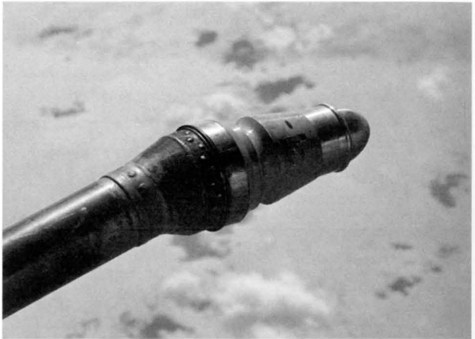
On the end of the KC-135 boom was a basket which went into an Omega shape, and this put more stress on the Lightning's connection. The weak link safety device just behind the nozzle in the probe, which broke off in emergency, was too weak to mate with the KC-135. Dick Bell
