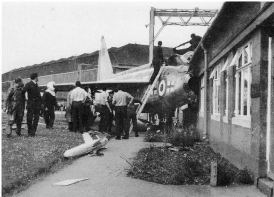
On 21 June 1968 Sqn Ldr Arthur Tilsley taxied in with no brakes and buried F.1A XM188 in the side of No.1 Hangar. Both engines jammed at about 80 per cent power and Chief Tech Brian Hayes, Propulsion Trade Manager, scrambled underneath to the engine bay and eventually managed to stop the engine. Arthur Tilsley (being led away, left of the picture) climbed out of the cockpit onto the roof of the hangar offices. via Jean Stangroom
