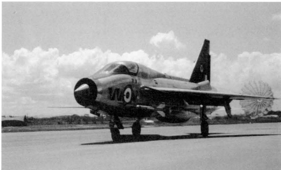
T.5 XV329 was sent by sea to Singapore from Sydenham, Belfast, in June 1967, when 74 Squadron deployed to Tengah from Leuchars. It returned by sea to the United Kingdom in August 1971, and had to be written off in December when it was discovered that acid spillage from the batteries had corroded the airframe. Gp Capt Dave Roome
