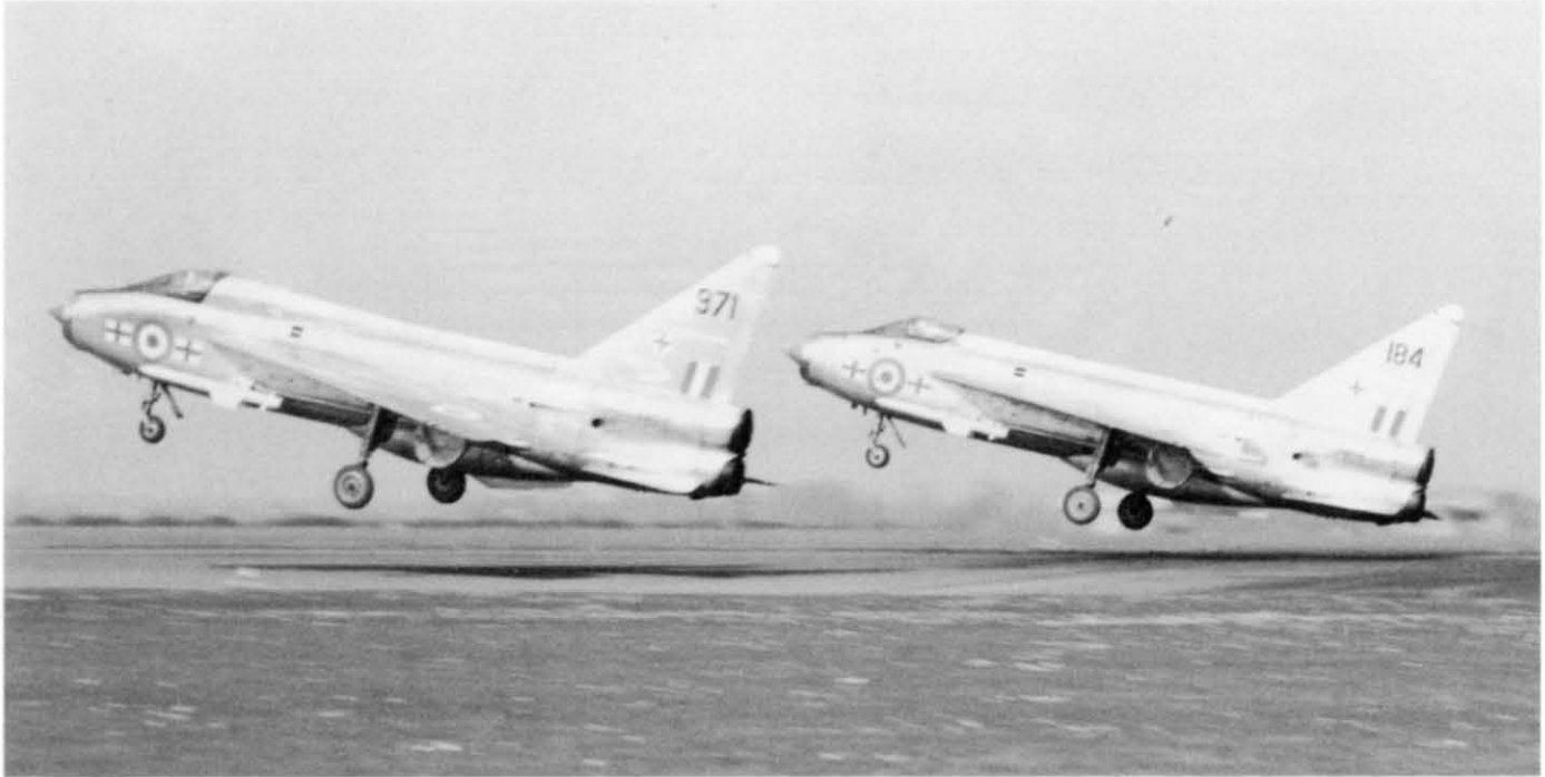
F.1A XM184 and T.4 XM971 taking off from RAF Coltishall. XM971 was lost on a dual radar sortie on 2 January 1967. Both Sqn Ldr Terry Carlton, OC No.2 Squadron, and his student, Flt Lt Lloyd Gross, ejected safely after the aircraft suffered an immediate loss of power caused by the radome coming loose and the debris being ingested by the engines. Gross ejected first, Carlton going at about 800ft, the aircraft crashing at Tunstead. Both pilots, each of whom suffered spinal injuries, were recovered by a Whirlwind from the SAR Flight of 202 Squadron on the base. While being flown by Flt Lt Gerry Crumbie, XM184 caught fire on landing on 17 April 1967 and had to be written-off. Crumbie was unhurt. Simon Parry
