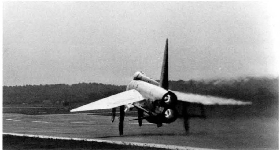
Due to the high fuel consumption when re-heat was used and the consequent reduction in total endurance, only one dual and one solo re-heat take-off and climb were carried out during OCU training. Fuel used on a re-heat climb only exceeded that used in a cold climb by a small margin. Distance to height was 28nm on cold power, and 16nm on re-heat; while time to height was 3fl minutes on cold power and 2fi minutes on re-heat. via Bruce Hopkins/Aeroplane
