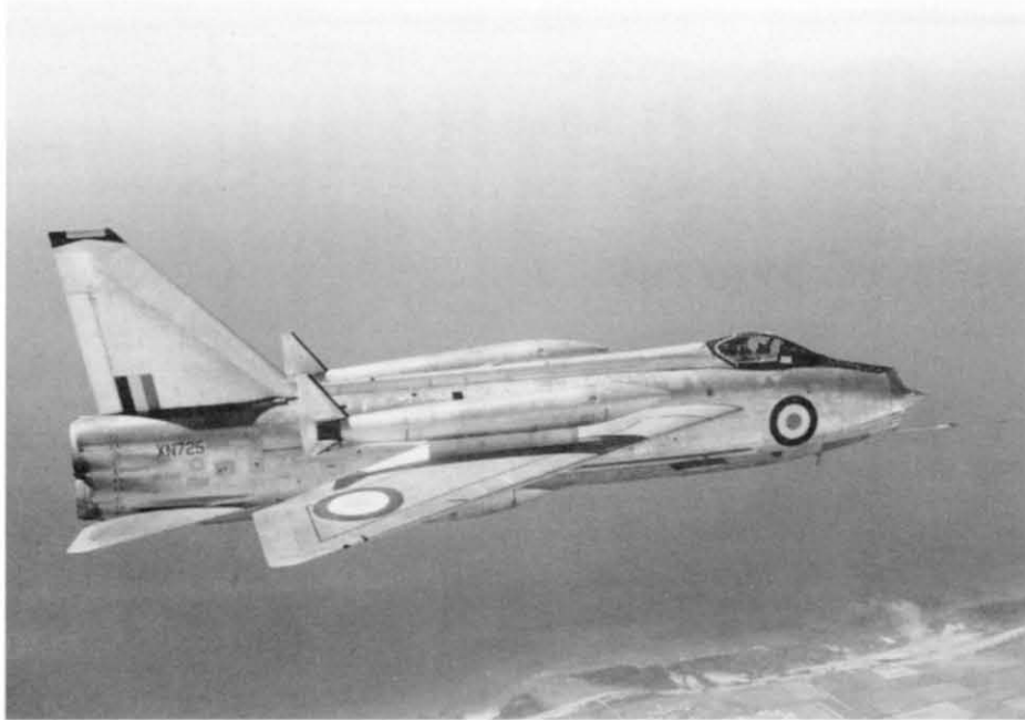
F.2 XN725 was one of a batch of forty-four built, the first to have a cambered wing, and was first flown on 31 March 1962 by Jimmy Dell. Seen here fitted with test overwing tanks, it was converted to the F.3 prototype and fitted with Avon 301 engines. It operated for a time at RAE Bedford for Concorde 'noise' and high-speed trials. BAe
