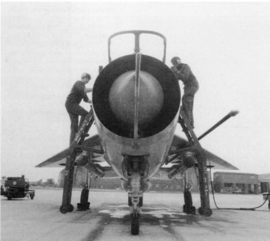
Two linies at work on a Lightning. An acquisition round is fitted to the port side only, no doubt because, with the rundown of the Lightning fleet, there were not enough to have more than one per aircraft. In earlier years the 'acqui' was always fitted to the starboard side so that if the aircraft went inflight refuelling there was no danger of the basket hitting and breaking the glass nose. A white painted metal flyable 'cap' over the missile seeker head was used during long transit flights, or when inflight refuelling was planned. MoD
