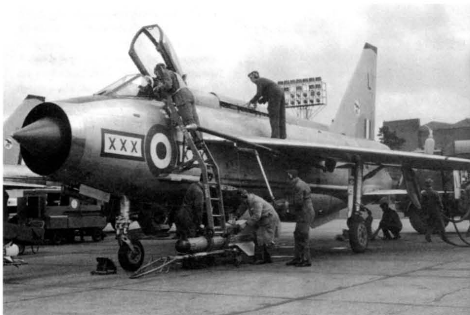
F.3 XP705/L of 29 Squadron being refuelled and rearmed at Wattisham on a practice operational turn-round in May 1968. Pete Nash works the winch while the other 'linies' go about their tasks. A hand brace was placed in the small hole just in front of the Ejector Release Unit (ERU) warning triangle, using the built-in winch to lower the missile pack. Whilst the ERUs were fitted, jettison cartridges were never fitted. If they were, the safety distances between aircraft would have meant that less than half of the slots on the pan could be used. Pete Nash
