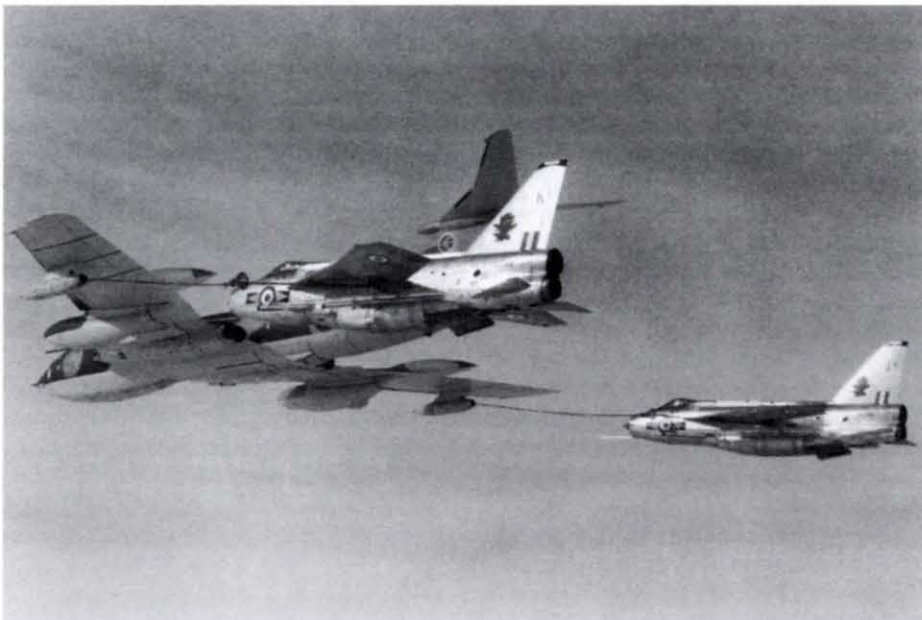
The Victor K.2 increased the fuel available to receiver aircraft. Here, a K.2 of 232 OCU at Marham refuels two F.6s of 11 Squadron, XR724/K and XR769/J, during an exercise in September 1974. MoD
