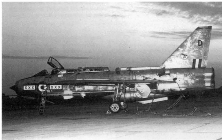
On its first flight at Wattisham after coming out of ASF, on 12 July 1972, F.3 XP694 of 29 Squadron suffered a double brake failure on landing and engaged the barrier. The top wire has taken off a small 'shark fin' aerial from the canopy and has ripped into the spine. Pete Nash
