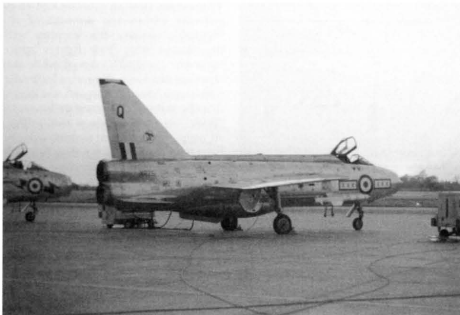
F.3 XR751/Q of 29 Squadron pictured at the southern, Bildeston end ORP (Operational Readiness Pan) during an air defence exercise in the early 1970s at Wattisham. The long thin cable snaking out to the starboard wheel-well is the 'telebrief', a landline through which the pilot could talk to the Station Operations and to Sector Control and receive his initial interception instructions and the order to 'scramble'. With the cockpit vacant it would indicate a low level of alert with possibly another Lightning on the line at cockpit readiness. On these exercises 29 and 111 Squadrons would share the same ORP; at other times each would be at opposite ends of the runway. Pete Nash
