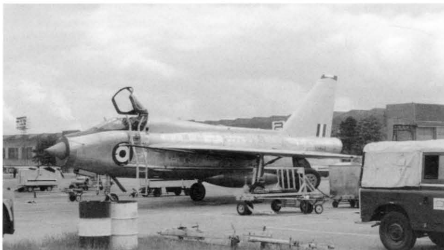
T.5 XS422 which served on 226 OCU at Coltishall from June 1965, is pictured newly arrived on 29 Squadron in 1972. The small square panel open behind the cockpit gives access to the canopy raise/lower switch and external locking handle. In the foreground are two 45-gallon drums, the red and white striped one for FOD (foreign object debris) and the white one filled with water to be used for dunking anyone caught by the ammonia. In the centre are two old-style towing arms, heavy and awkward to use (later replaced by a NATO standard lightweight towing arm). The tilt on the Land Rover is painted yellow so that it can be seen by Air Traffic Control. The flat top trolley contains a main-wheel jacking adaptor, a bottle jack, two brake units, a nose-wheel and four main wheels. The small box contains a supply of split pins. Behind the wheel trolley is the canvas-sided brake 'chute trolley. The steps at the back of the aircraft are being used by a rigger to fit the cable for the brake 'chute in clips around the jet pipes. If he is following the normal practice he has climbed the steps until halfway and then stepped onto the starboard tailplane. XS422 was transferred to 56 Squadron in 1973 and later served with the ETPS at Boscombe Down. Pete Nash
