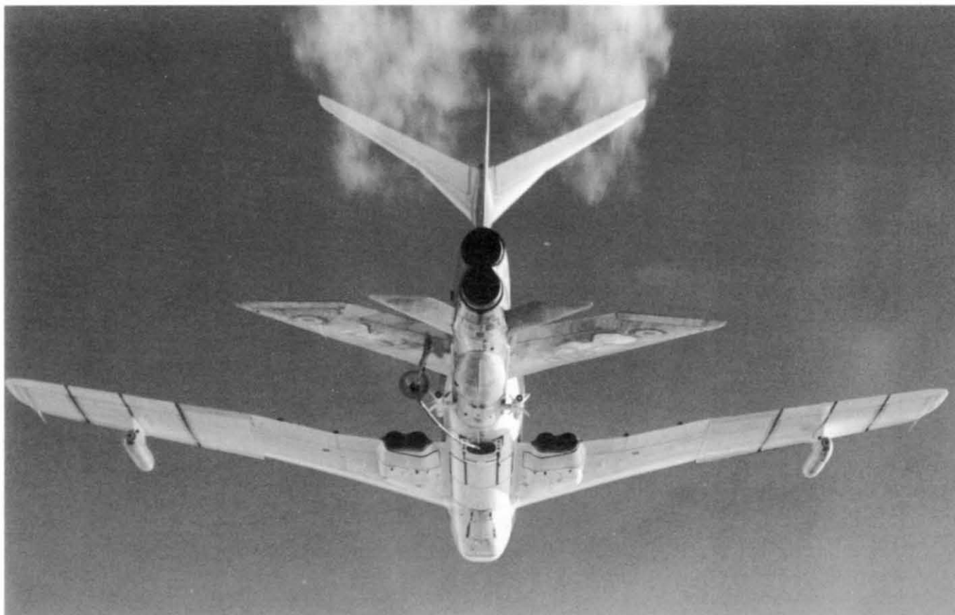
Normally, Lightning pilots tanked from the Victor's wing positions, the rear, central position only being used by the bigger aircraft. In this photo F.3 XP747/S of 29 Squadron uses the central position on Victor K.1A XA932. XP747 had operated with 56 Squadron until it suffered Cat.4 damage on 11
