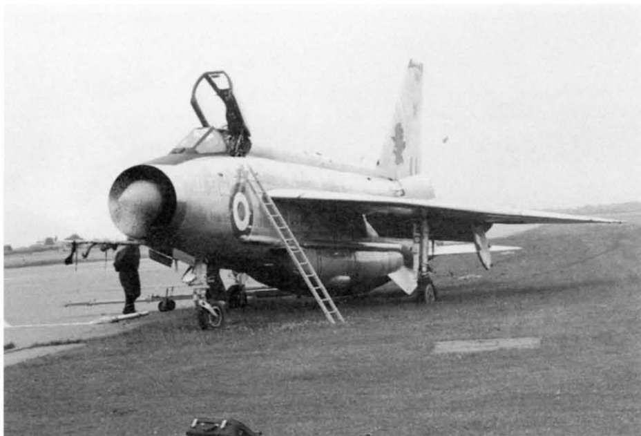
F.6 XR724 of 11 Squadron was being flown for the first time following a major servicing by Sqn Ldr Dick Bell, a Leconfield test pilot, on 28 July 1972, when it suffered a fire in the No.1 engine which was caused by a hydraulic coupling not being tightened up sufficiently. The fire went out but the F.6 was heavy and the pilot had a 185kt threshold speed. There was no wind and no parachute. Dick Bell rejected the early hookwire so that the aircraft would not be stretched and was aiming for the far hookwire relying on brakes when the port tyre burst. Despite full maxarats on full right rudder he could not control it and he had to heave the aircraft onto the grass where it stopped. Dick Bell
