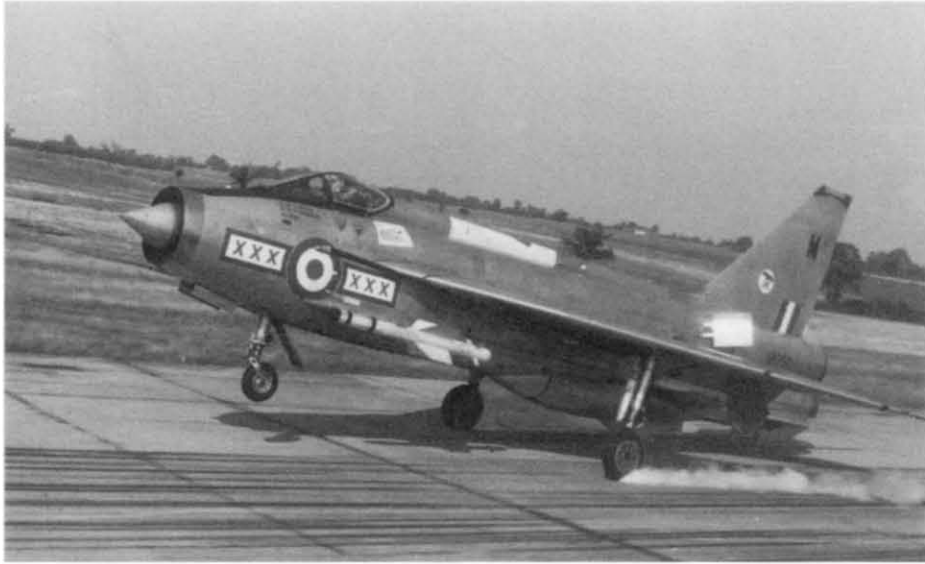
Good tyres were important; at fifteen tons the Lightning landed at about 140kt on tyres about six inches wide and inflated to 345 psi. They only lasted for seven landings, and many times less than that. For this reason, the Lightning never did a 'roller' touch and go landing. The ONLY time a Lightning took off again after touching down was on the rare occasions that the brake parachute 'candled'. Dick Bell
