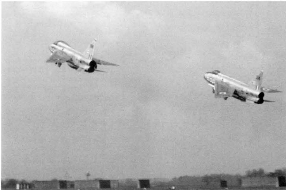
After lift-off, there was a gentle lurch forward as the main legs unlocked and retracted backwards and outwards into the sixty-degree swept wings. Their hinge axes were cleverly angled to achieve the desired orientation of the wheel. The nose leg, retracting against the airflow, took longer to lock up. The aircraft, climbing at about ten degrees, quickly accelerated to its normal climbing speed of 450kt IAS (not much has ever matched that!) by which time the pilot would have eased the nose up to about twenty-two degrees.
