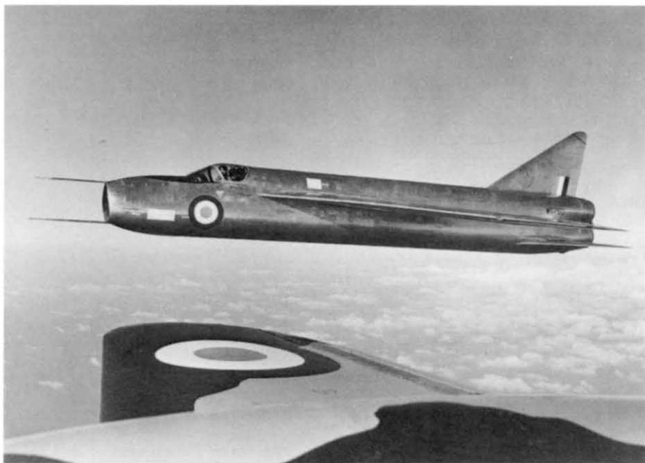
Air-to-air view of WG760 in the hands of Roland Beamont, taken by Charles E. Brown from a Gloster Meteor. The P.1A's leading edge chord-wise slot is very visible. Aeroplane
