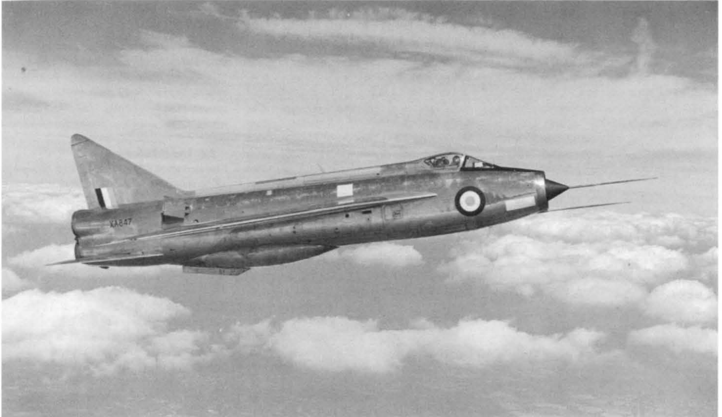
XA847, first of the three P.1B prototypes, which first flew on 4 April 1957 in the hands of 'Bee' Beamont. On 25 November 1958 it became the first British aircraft to fly at Mach 2. The Lightning, when it came into service in 1960, doubled the performance of the then-best RAF fighter (The Hunter) in front-line service. It was lightly armed, with only two Firestreak air-to-air infra-red guided weapons and two Aden cannon, but its ability to manoeuvre with the best and out-climb all of them gave its pilots an advantage which set them apart from others. The F-104 Starfighter had, eventually, the same straight-line top speeds but could never match the Lightning's rate of turn at any speed. It was not until the F-15 came along fifteen years later that the Lightning had any real competitor. Aeroplane
