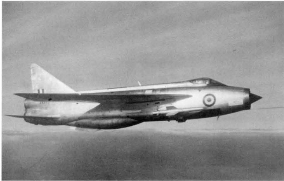
NS853, the second of the three P.1B prototypes, which was flown for the first time by D. de Villiers on 5 September 1957. Mostly it was used on gun trials and gas-concentration tests. It lost its fin during an accidental canopy ejection and on its fifty-first flight test pilot Jimmy Dell suffered an in-flight fire. via Ray Biddle
