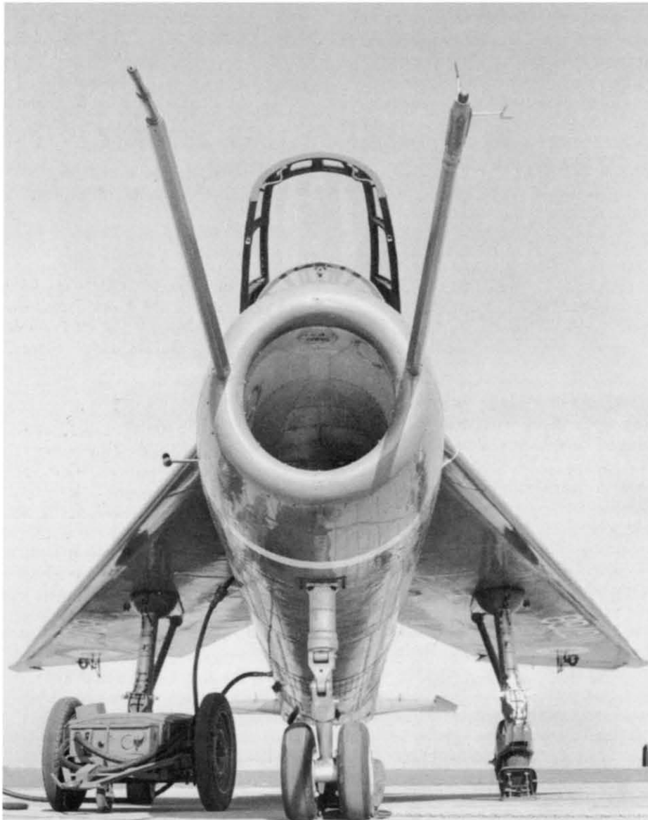
English Electric were helped greatly in the development of the P.1 by data provided by WG768, the Short SB.5, a scaled down test-bed powered by a 3,500lb (1,600kg) thrust Rolls-Royce Derwent and fitted with a non-retractable undercarriage, adjustable for centre of gravity variations. The SB.5 first flew on 2 December 1952. Aeroplane
