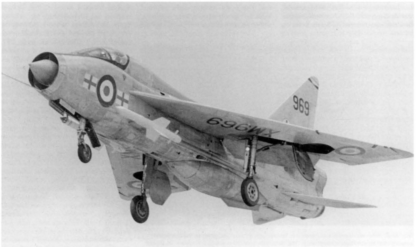
Handling the aircraft at Mach 0.95 was practised during the first conversion exercise and would normally consist of the student getting the feel of the controls. A speed of Mach 0.95 was chosen as this was the best subsonic manoeuvring speed. Ronald Johnson
