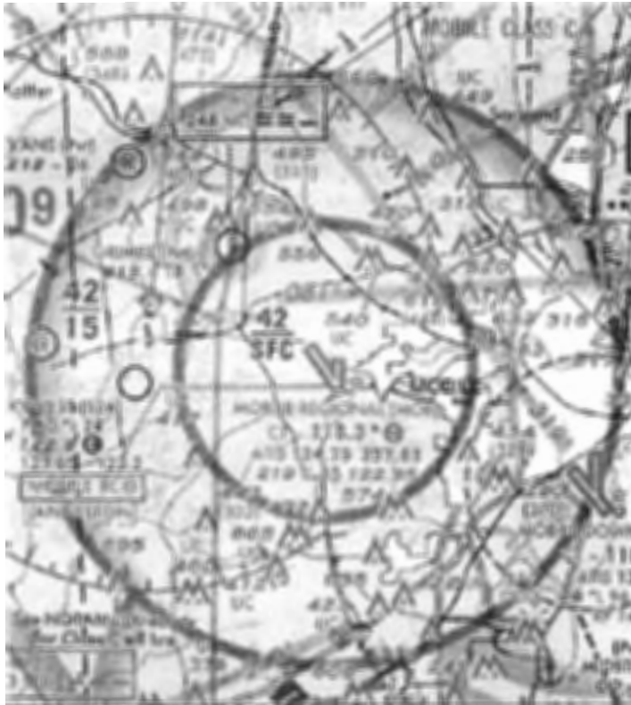
Figure 5-7. Class C airspace surrounding Mobile, Alabama, International Airport. (Source: National Aeronautical Charting Office, FAA) (Not for navigational use)
