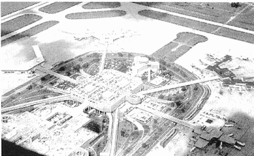
Figure 7-11. Example of airside-landside concept, Tampa International Airport. (Figure courtesy Hillsborough County Airport Authority)
