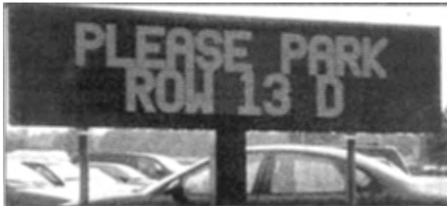
Figure 7-31. Smart parking facilities provide specific parking space availability.
