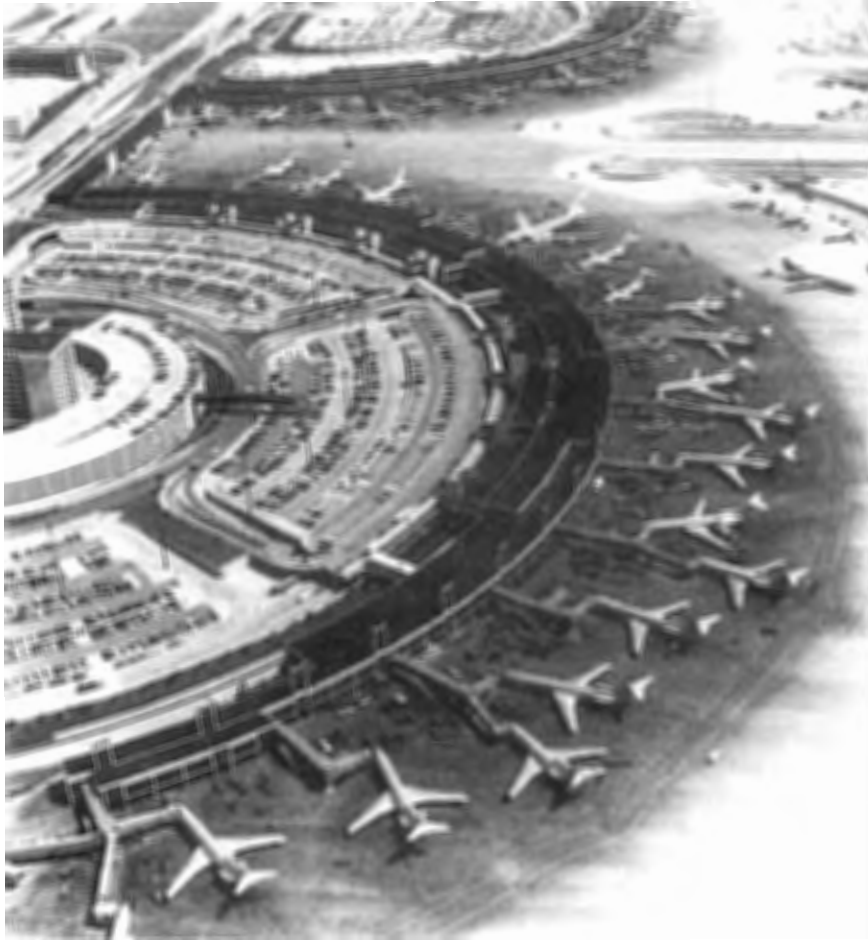
Figure 7-5. DFW Airport, whose terminal area employs a multiple-unit curvilinear terminal concept, now accommodates a large percentage of transfer passengers. (Photo courtesy FAA)
