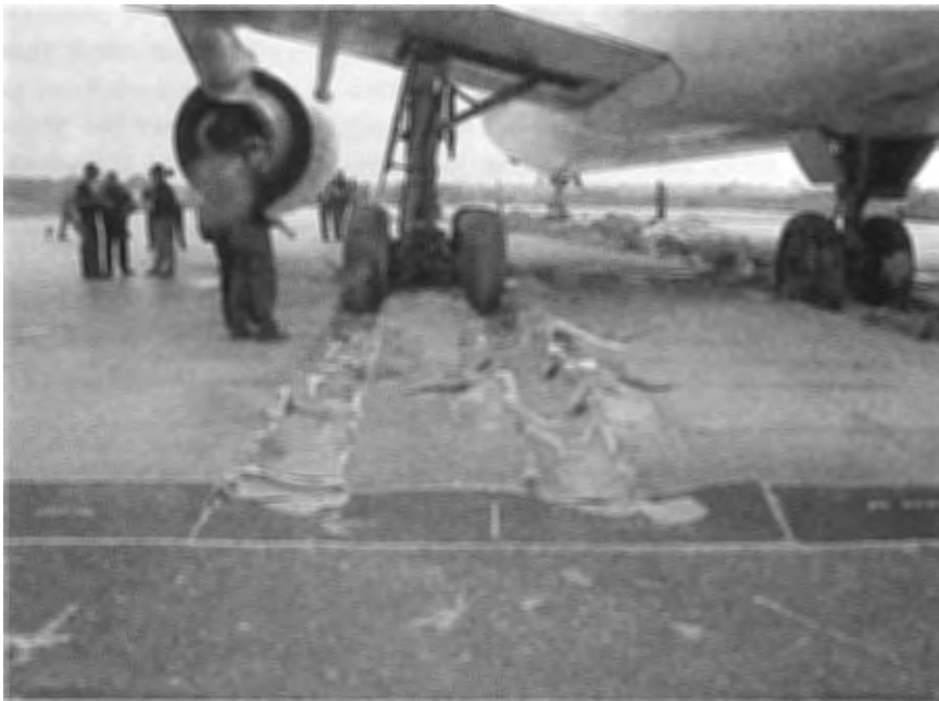
Figure 4-10. EMAS system at New York’s John F. Kennedy International Airport. (Figure courtesy Port Authority of New York and New Jersey)
