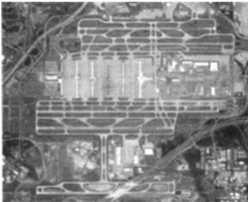
Figure 4-3. Atlanta's Hartsfield International Airport has five primary parallel runways to accommodate high-volume large-aircraft operations. (Courtesy Google maps)
