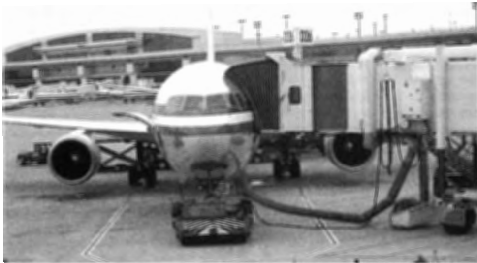
Figure 7-15. Loading bridges are part of the flight interface. (Picture courtesy Dallas Regional Chamber)
