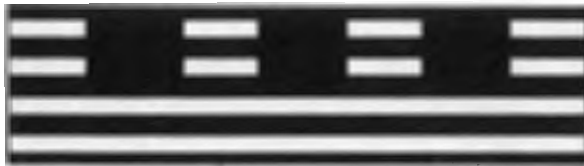
Figure 4-13. Runway holding position markings, yellow markings on black background.
