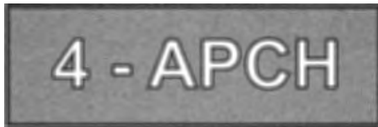
Figure 4-23. Runway approach area holding sign. (Source: FAA AIM)
