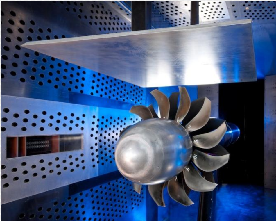
Figure 9.1: Model scale cruise simulations in the NASA Glenn 8' x 6' Supersonic Wind Tunnel with acoustic plate installed for near field noise assessments.
