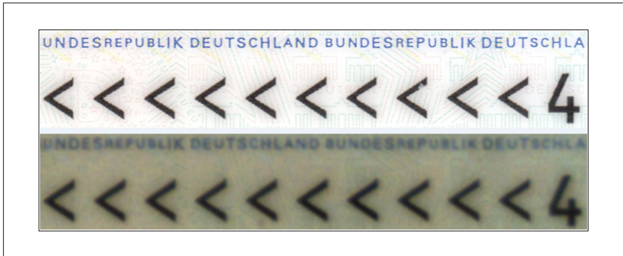
Figure C-9. Passport (D, P, 1, 2017): Comparison between a high-resolution image of the microtext (1000 ppi) and an image of the same microtext taken from a full page reader (nominal 400 ppi)
