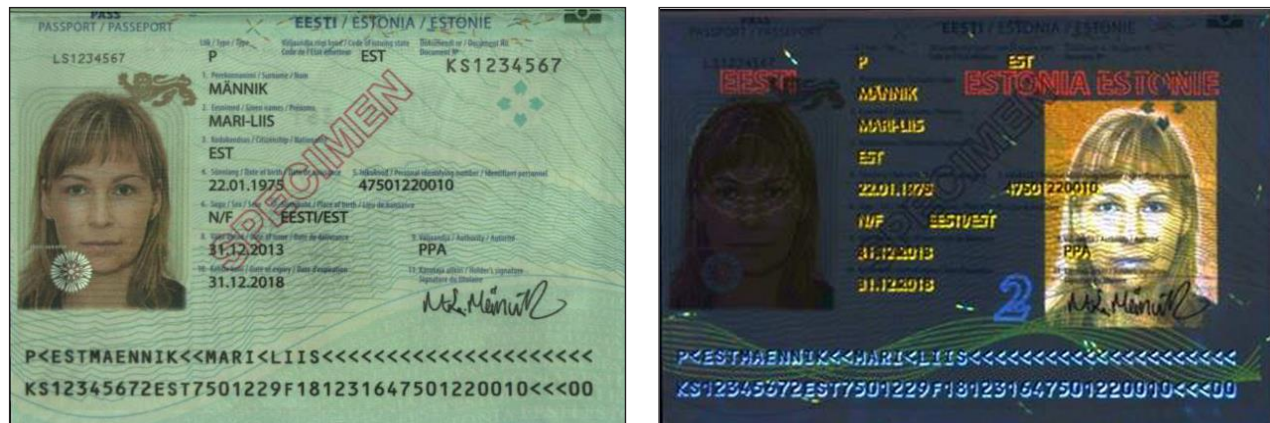
Figure C-12. Passport (EST, P, 1, 2013): Verify the facial image in the visible light image against the one printed with UV luminescent ink
