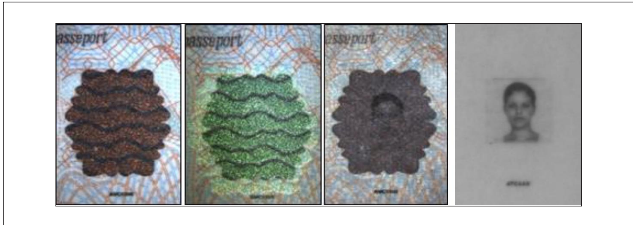
Figure C-6. Passport (HUN, P, 1, 2006): Personalized OVI viewed under two different angles under transmitted light and under IR light
