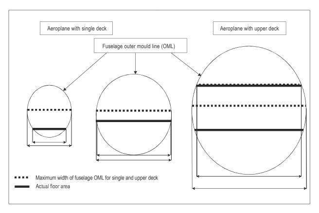
Figure A2-1. Cross-sectional view
