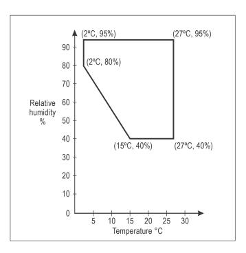
Figure A6-2. Measurement window for no absorption correction
