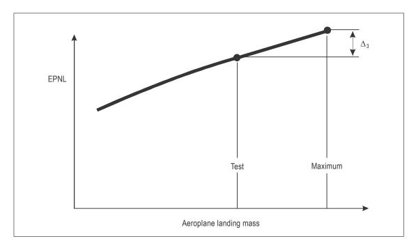
Figure A1-11. Approach mass correction for EPNL
