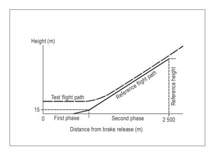
Figure A6-1. Typical test and reference profiles
