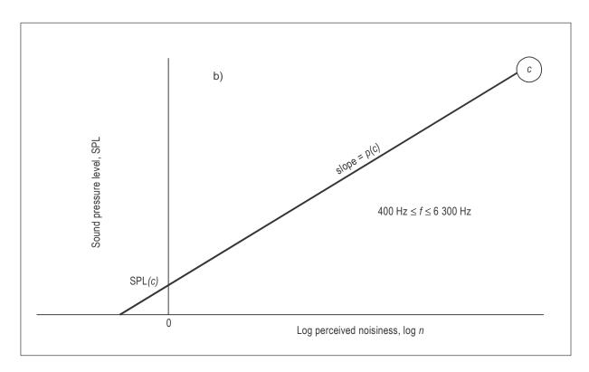
Figure A1-3. Sound pressure level as a function of perceived noisiness
