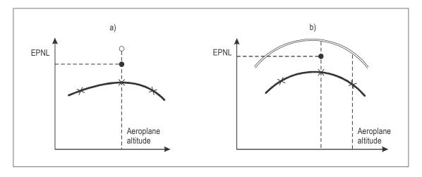
Figure A2-13. Lateral asymmetry adjustments
