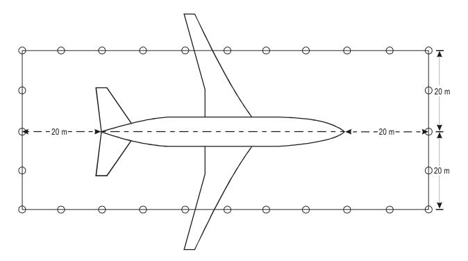
Figure C-2. Rectangle of noise survey measurement positions
