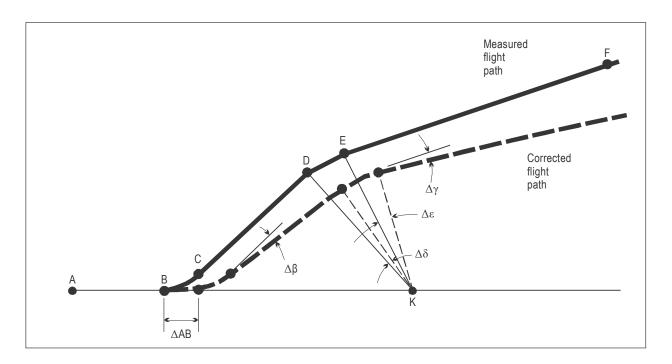
Figure A1-5. Comparison of measured and corrected take-off profiles
