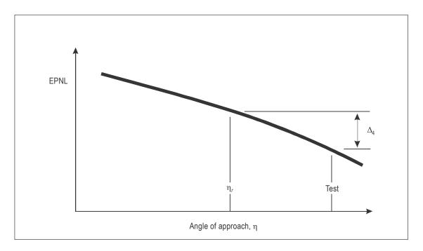
Figure A1-12. Approach angle correction for EPNL
