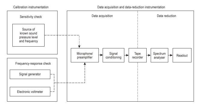
Figure C-1. Noise measurement systems
