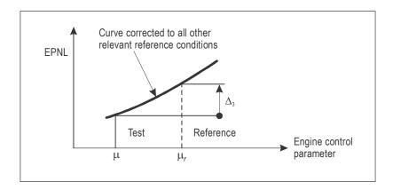
Figure A2-12. Source noise adjustment
