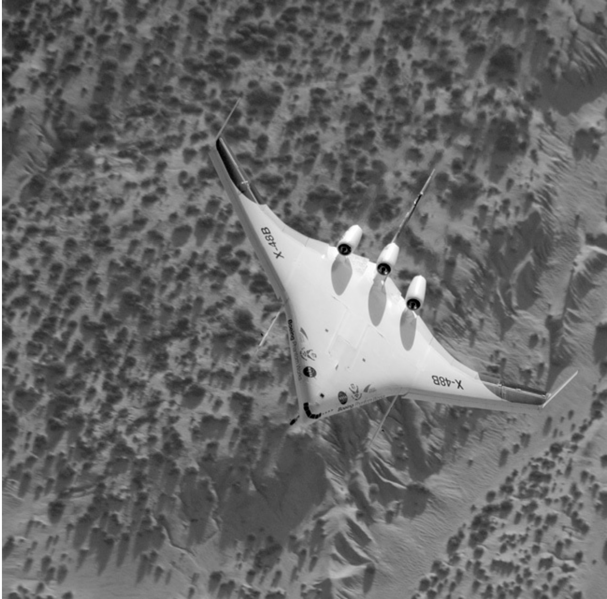
Figure 1-5. NASA is currently researching a blended wing body design for quieter and more efficient transport category jets. Here, a subscale X-48B is seen banking over desert scrub at Edwards Air Force Base. (NASA photo)
