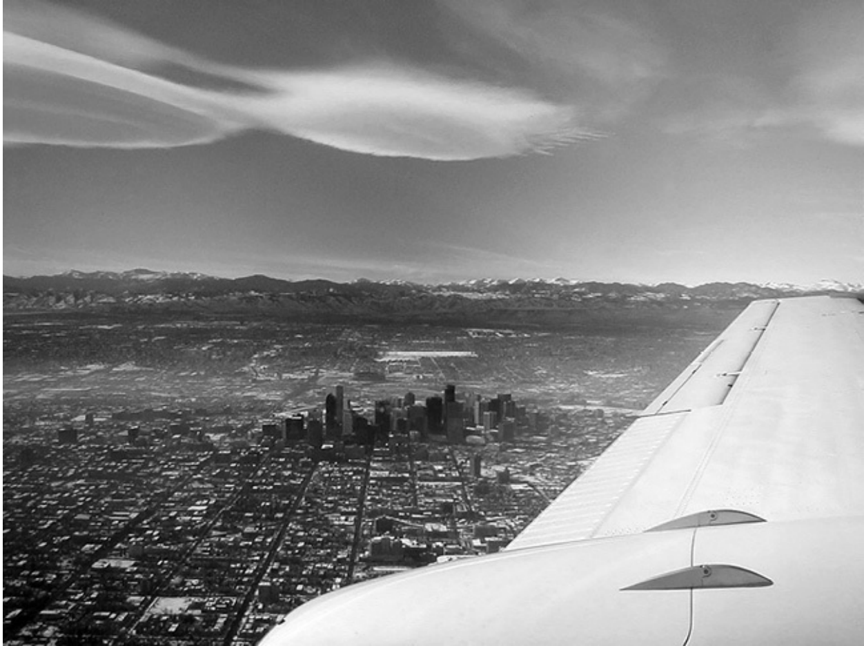
Figure 8-3. Lenticular (lens-shaped) clouds over Denver warn of clear air turbulence over and east of the Rockies. ( Photo by Bernie Roland )
