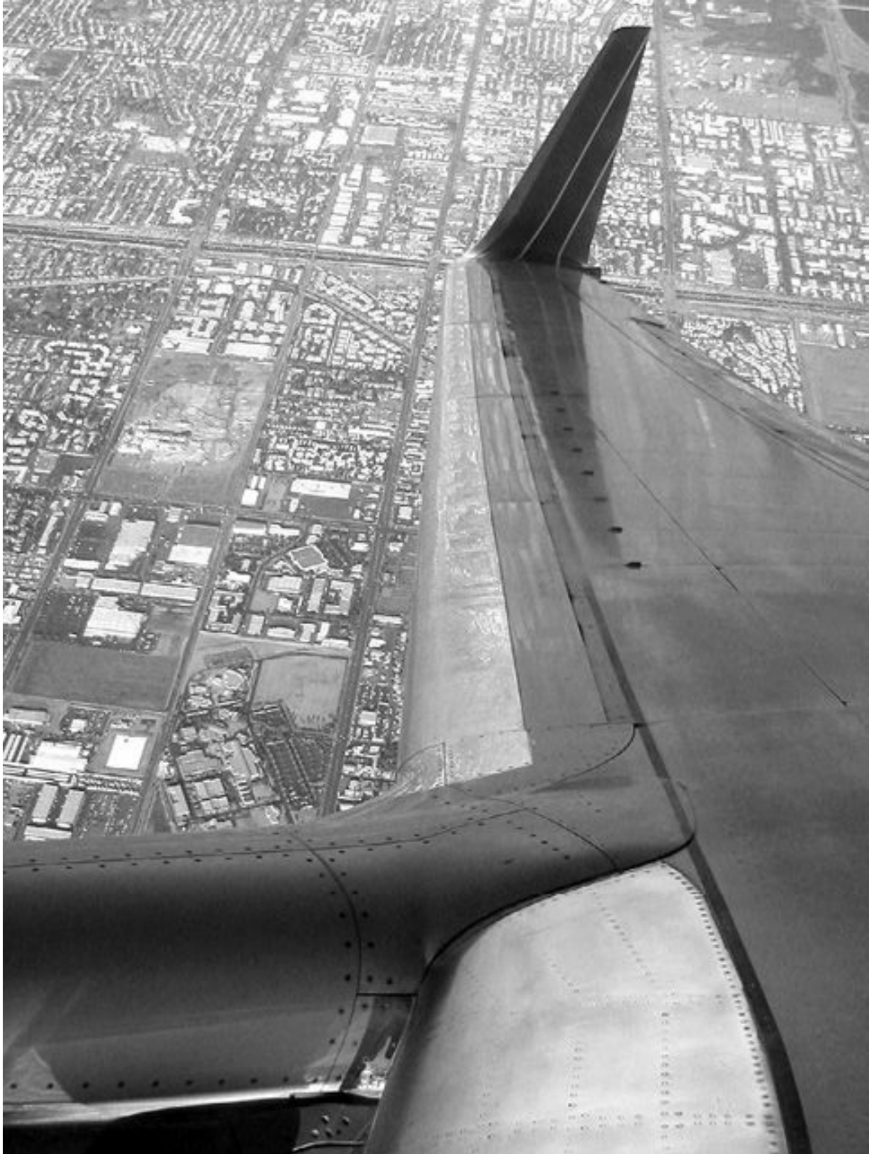
Figure 1-4. Many airliners are sprouting winglets such as these, originally
