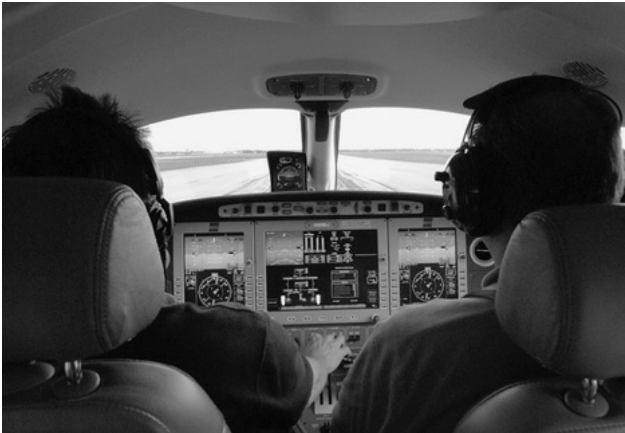
Figure 1-6. The ergonomically designed high-tech “glass cockpit” in this very light jet (VLJ) exemplifies the ease of operation goals of the AGATE and SATS
