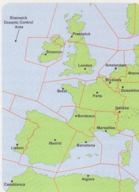
Figure 5.2 All Airspace belongs to some specified Flight Information Region (FIR). Oceanic Airspace is divided into Oceanic Information Regions.
