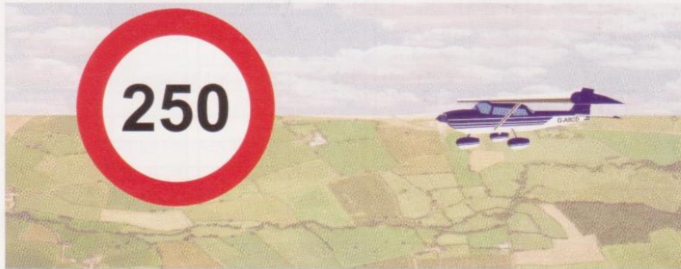
Figure 2.29 The Rules: Generally an aircraft shall not fly faster than 250 kts IAS below 10 000 feet unless cleared by ATS.
