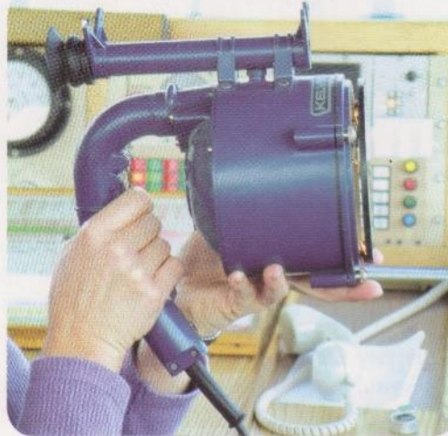
Figure 9.3 A signalling lamp.
