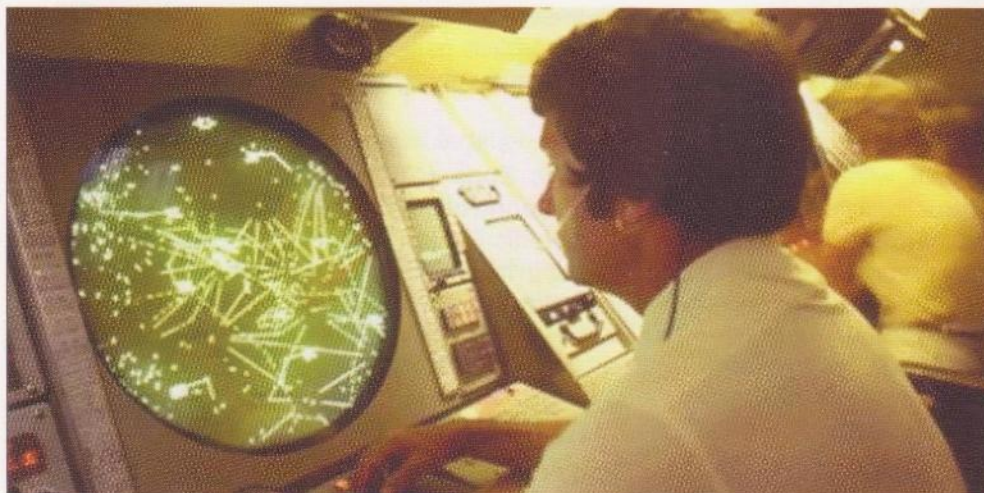
Figure 5.17 Approach Control Unit.
