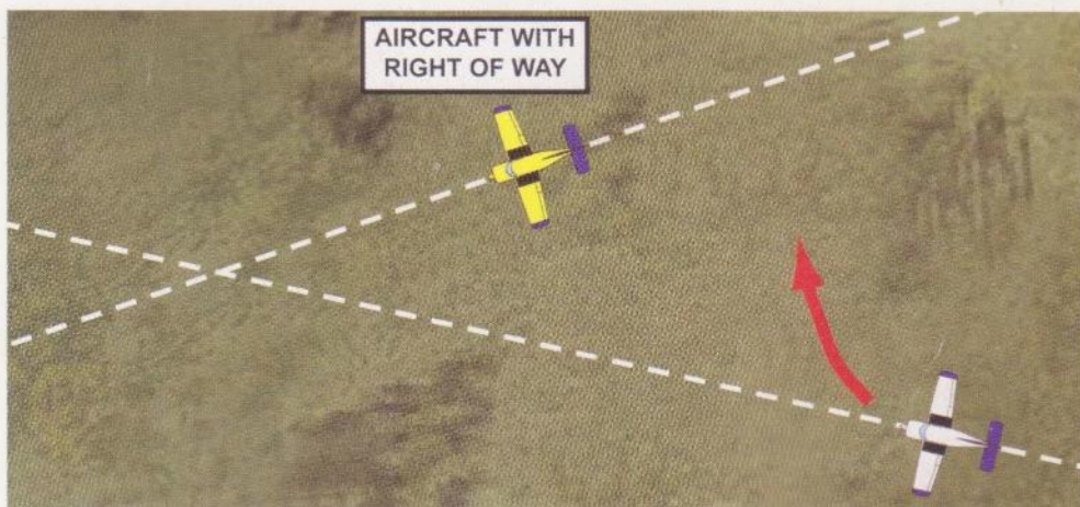
Figure 2.12 An aircraft giving way must avoid passing over, under or in front of the aircraft with right of way.
