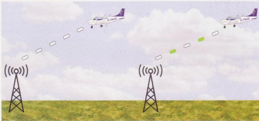
Figure 9.15 Aerodrome beacons flashing either white, or green and white.
