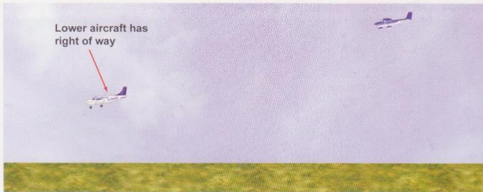
Figure 2.11 Right of Way on Landing. The lower aircraft has right of way.
