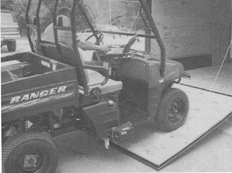
Figure 5-16. Lightweight Profiler (Dynatest 2004).
