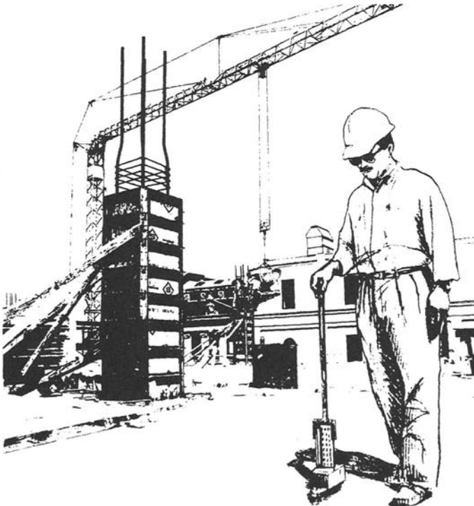
Figure 5-17. Dipstick Auto-read Profiler (FACE 2004).
