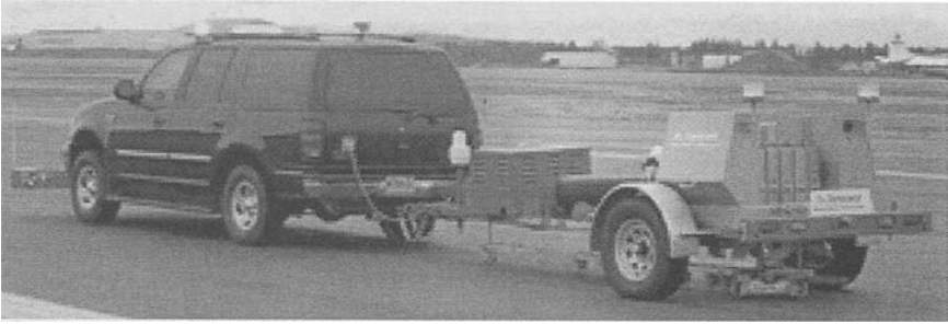
Figure 4-2. Heavy Dynatest FWD (HWD).
