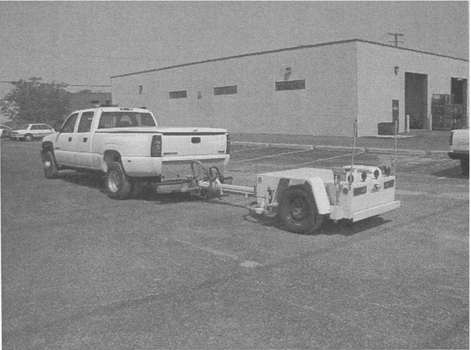
Figure 6-11. Locked-wheel Skid Trailers (Dynatest 2004).
