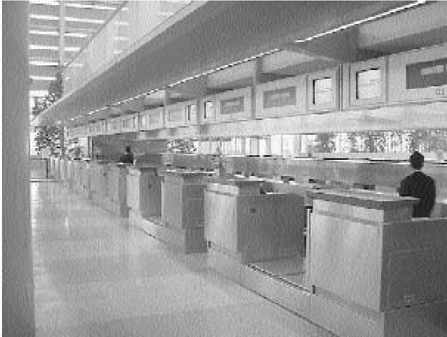
Figure 6-16. CUTE (common-use terminal equipment) with variable LED and CRT signage.
