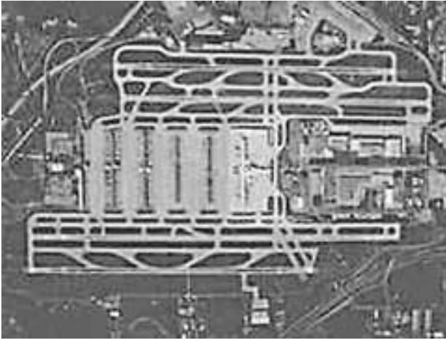
Figure 4-3. Atlanta's Hartsfield International Airport has two sets of parallel runways to accommodate high-volume large-aircraft operations. (Courtesy Hartsfield Atlanta International Airport)
