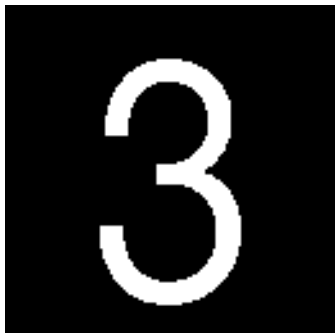
Figure 4-35. Runway distance remaining sign.
