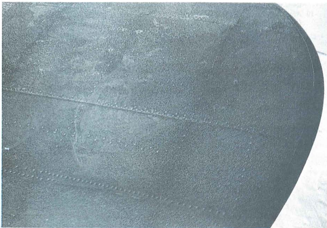
FIGURE 99. Frost on an aircraft. Always remove ice or frost before attempting takeoff.
