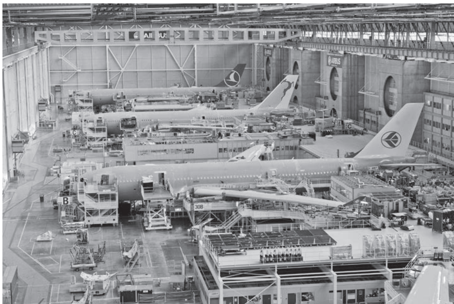
Figure 14.2 The A330 final assembly line at Toulouse, France, showing three aircraft at different stages of final assembly
